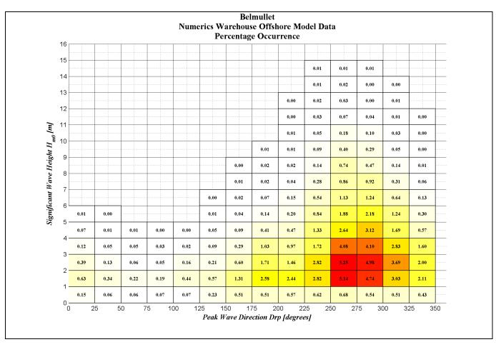
Figure 3.3 Offshore Hs/Wave Direction Scatter Diagram
