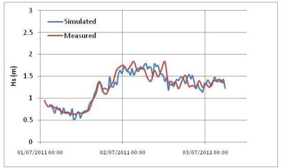
Figure 3.11  $H_s$  calibration curves for 'shallow' ADCP location
