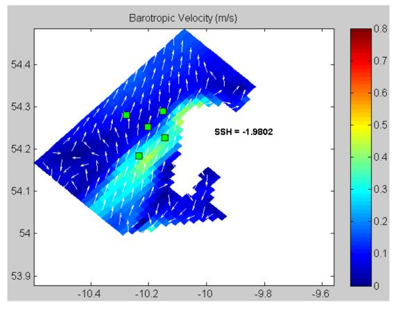
Figure 4.4 Tidal Flows from model output
