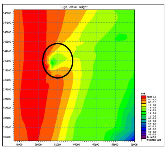
Figure 3.23 Impact of WECs on wave field at Test A
