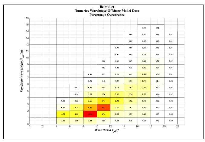
Figure 3.4 Offshore Hs/Tp Scatter Diagram
