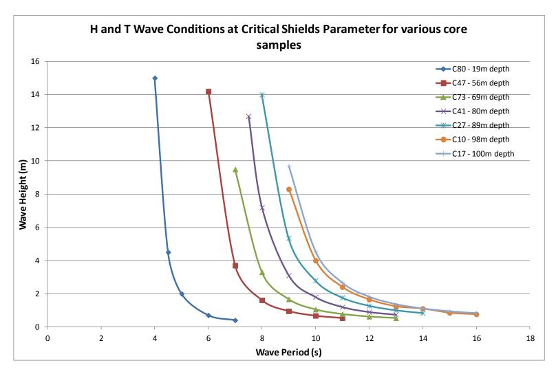
Figure 5.2 Critical Sediment Transport Conditions for each core sample
