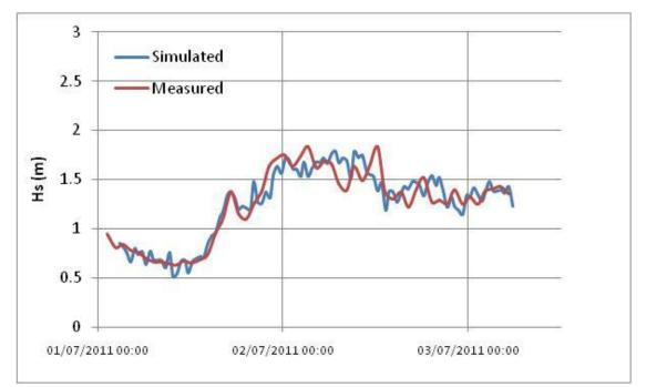
Figure 3.9 H<sub>s</sub> calibration curves for Test Area B ADCP location
