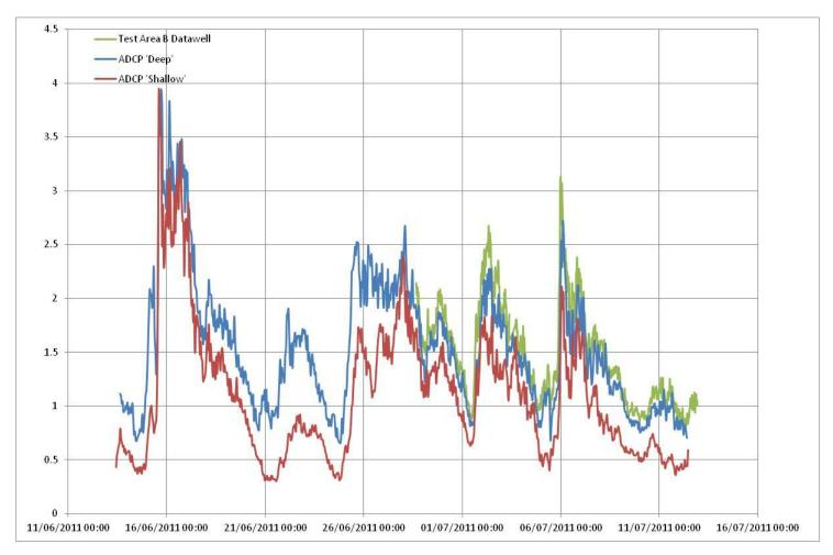
Figure 3.6 Coincident H<sub>s</sub> Measurements
