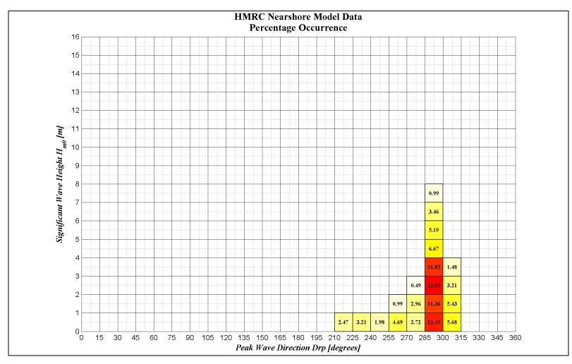
Figure 3.14 PT2 Hs/Wave Direction Scatter Diagram
