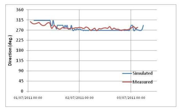
Figure 3.12 Wave Direction calibration curves for 'shallow' ADCP location
