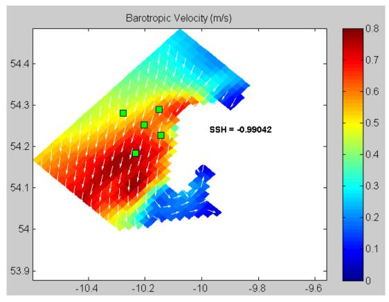
Figure 4.3 Tidal Flows from model output
