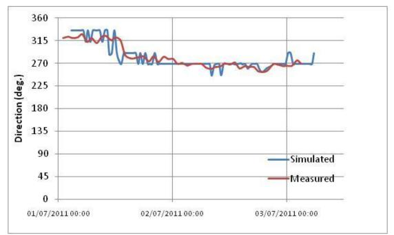
Figure 3.10 Wave Direction calibration curves for Test Area B ADCP location
