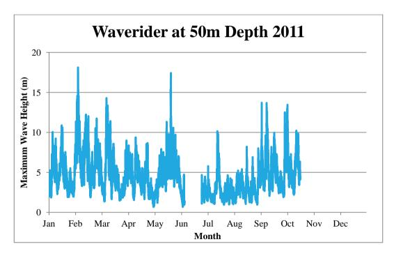
Figure 20 Distribution of maximum wave heights recorded by Belmullet Waverider at 50m depth (Test Area B) during 2011
