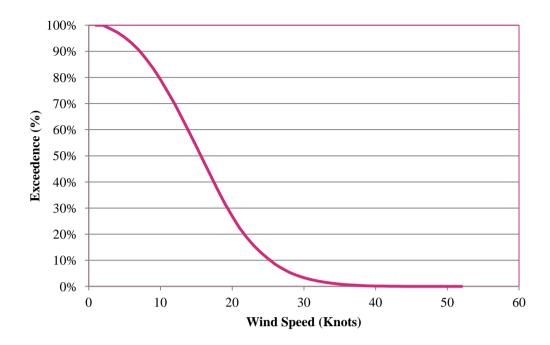
Figure 12 Weather Buoy M4: Wind Speed Exceedence Curve (2001 – 2010)
