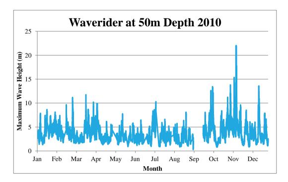
Figure 19 Distribution of maximum wave heights recorded by Belmullet Waverider at 50m depth (Test Area B) during 2010
