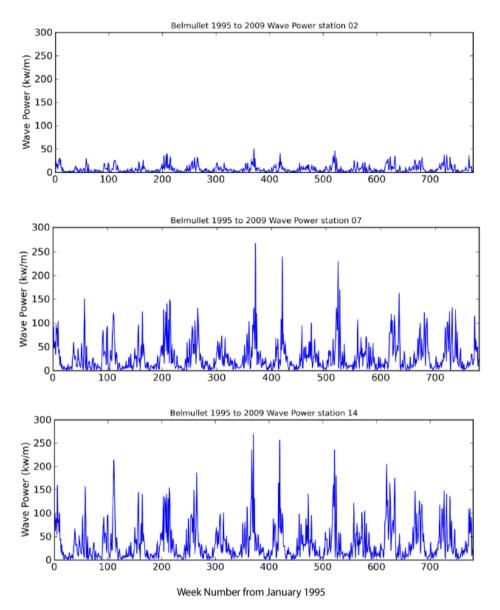
Figure 22 Omni-directional wave power weekly averages for selection of stations at different depths.
