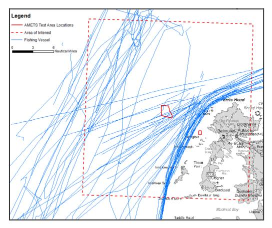
Figure 59 Winter Survey – fishing vessel tracks from radar & AIS data
