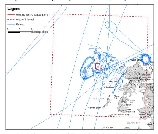
Figure 61 Summer Survey – fishing vessel tracks from radar & AIS data
