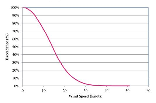
Figure 11 Weather Buoy M1: Wind Speed Exceedence Curve (2001 – 2007)
