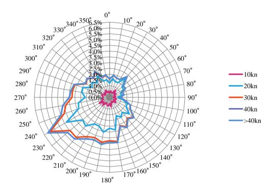
Figure 10 Weather Buoy M4: Wind Rose (2001 – 2010)
