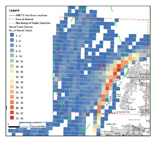
Figure 46 Vessel Track Density during the Winter Survey
