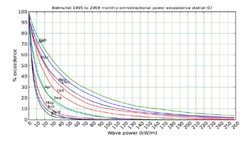
Figure 24 Percentage exceedence of wave power displayed by month for a recording station for the period 1995 to 2009.
