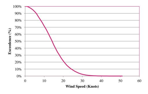
Figure 14 AMETS Buoy: Wind Speed Exceedence Curve (20/5/2010 – 7/10/2010; 24/3/2011 – 24/8/2011)
