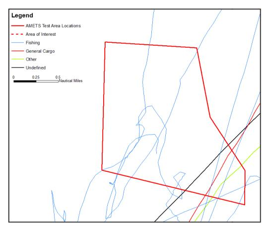
Figure 54 Summer Survey - detailed chart of tracks by vessel type passing within AMETS Test Area A.
