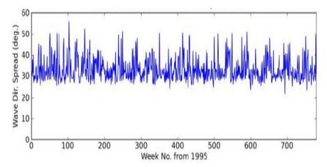
Figure 21 Standard deviation of wave directions recorded at station 07
