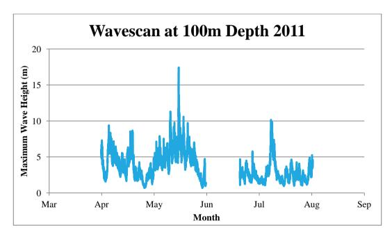
Figure 18 Distribution of maximum wave heights recorded by Belmullet Wavescan at 100m depth (Test Area A) during 2011
