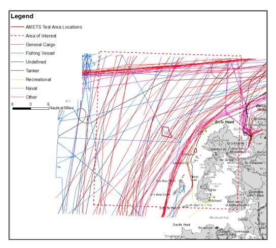
Figure 68 July 2010 AIS Tracks colour-coded based on Vessel Type
