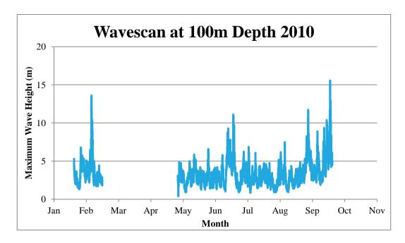
Figure 17 Distribution of maximum wave heights recorded by Belmullet Wavescan at 100m depth (Test Area A) during 2010
