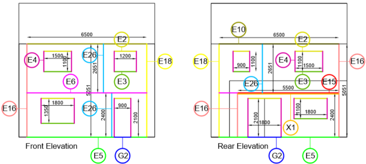
Figure 6.27: Elevations with all junctions identified
