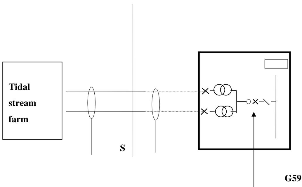
Fig.A6 Stream Farm to PES Network - basic arrangement
