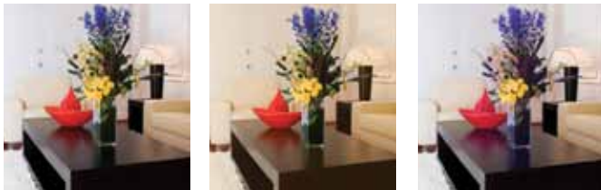
Fig. 2: Colour rendering characteristics of 3 different light sources (a) Daylight= Ra 100, (b) Tungsten = Ra 100, (c) Single phosphor cool 'white'= Ra 58.
