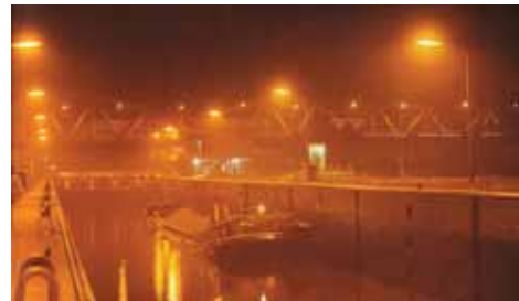
Fig. 3: Low pressure sodium lamps with poor colour rendering.
