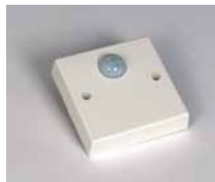
Fig.4 Infra-red wall sensor – Detects presence (in a range of 5 to 9 metres) and daylight – This 'No neutral' type can directly replace a standard manual switch.
