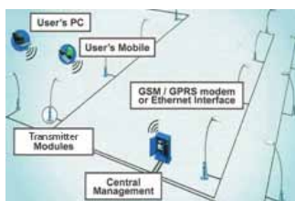
Fig. 5 Each component in a GPS networked control system and how they interface
