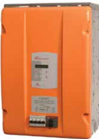
Fig. 4 Voltage control unit, Lighting Energy Controller (LEC) Type A, voltage supplied to the lighting circuits can be reduced up to 35V, in decrements of 2.5V.
