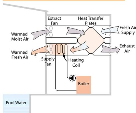
In the case of Finglas Swimming Pool there is a low level warm air supply via a concrete plenum on one side of the wall, with a mid height warm air supply via concealed ductwork on the other side of the wall. The hall extract is via two high level ducts on both sides of the walls.
