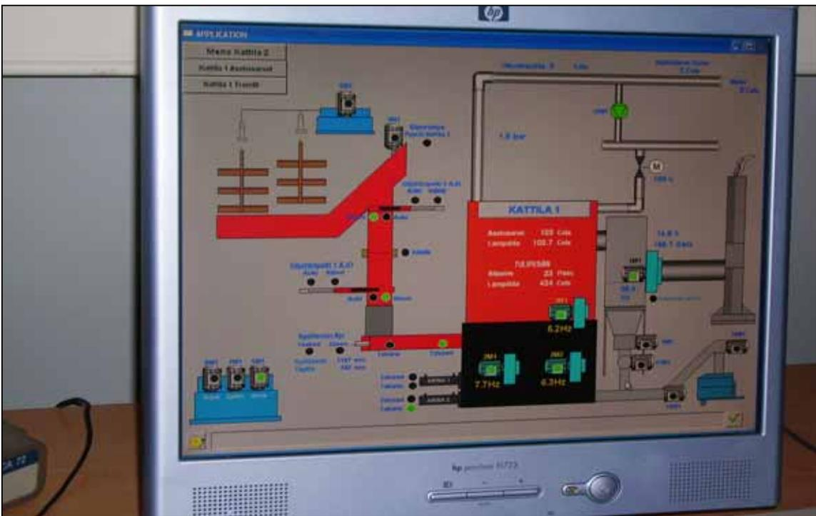
Fig 10. Computer control panel for heat plant accessible via the internet.
