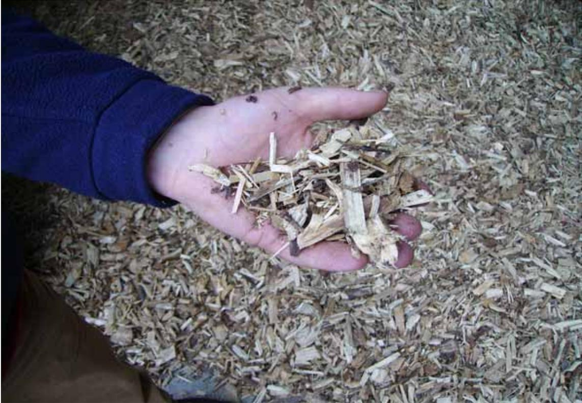
Fig 9. Sample of wood chips used in district heating plants.
