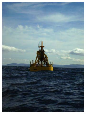
Figure 4-15: Quarter scale Wavebob WAB-PA device
