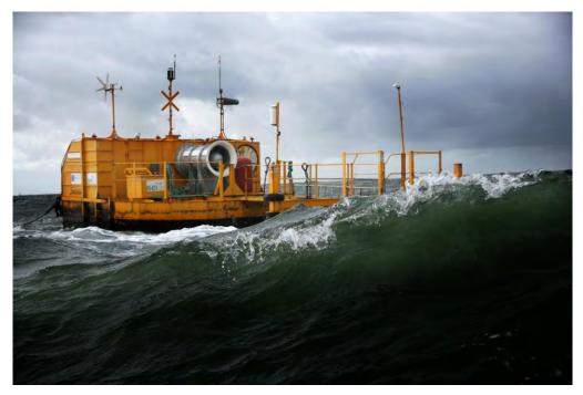
Figure4-16 : Quarter scale Ocean Energy OWC device
