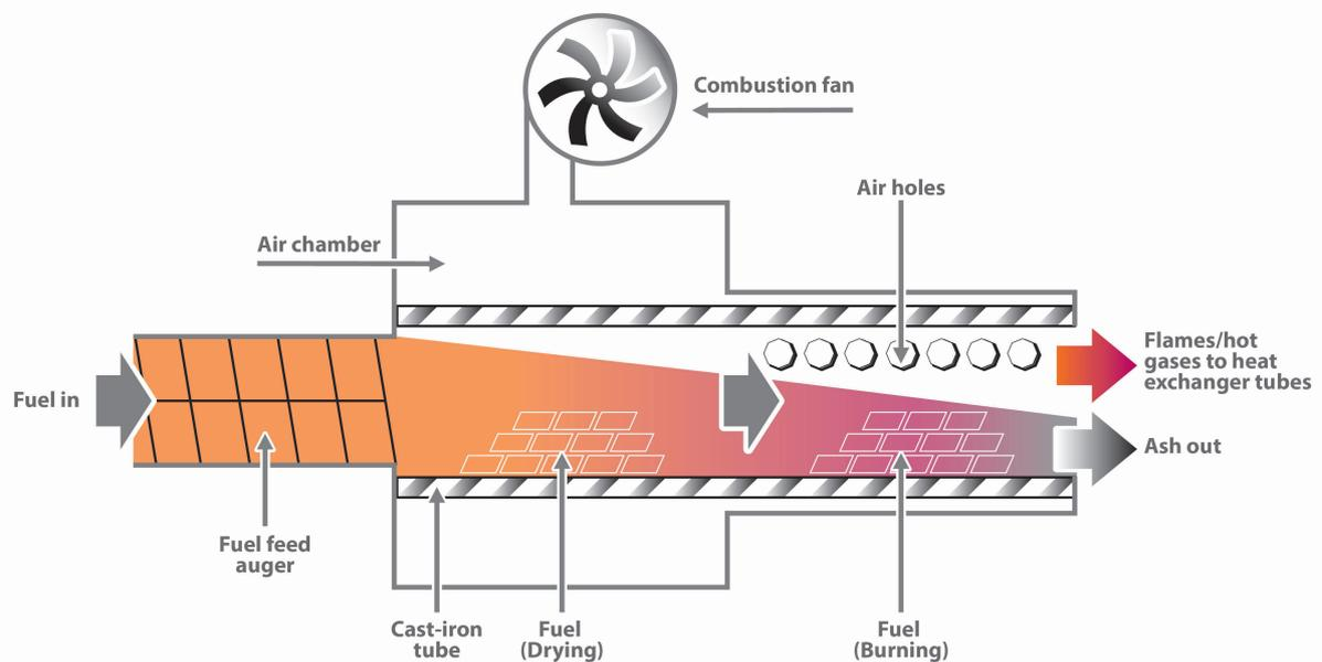
Figure 3.3: Small stoker burner boiler
