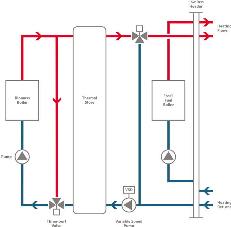
Figure 4.2: Biomass boiler and its thermal stored connected in series with fossil fuel boiler
