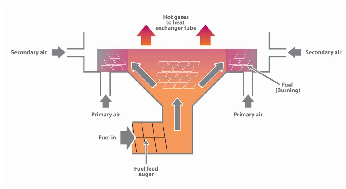
Like the stoker burner design, the low refractory mass (low thermal mass) and low fuel inventory mean that these boilers can respond rapidly to changes in heat demand. Most underfed stoker designs have separate primary and secondary combustion air fans, aiding complete combustion.
