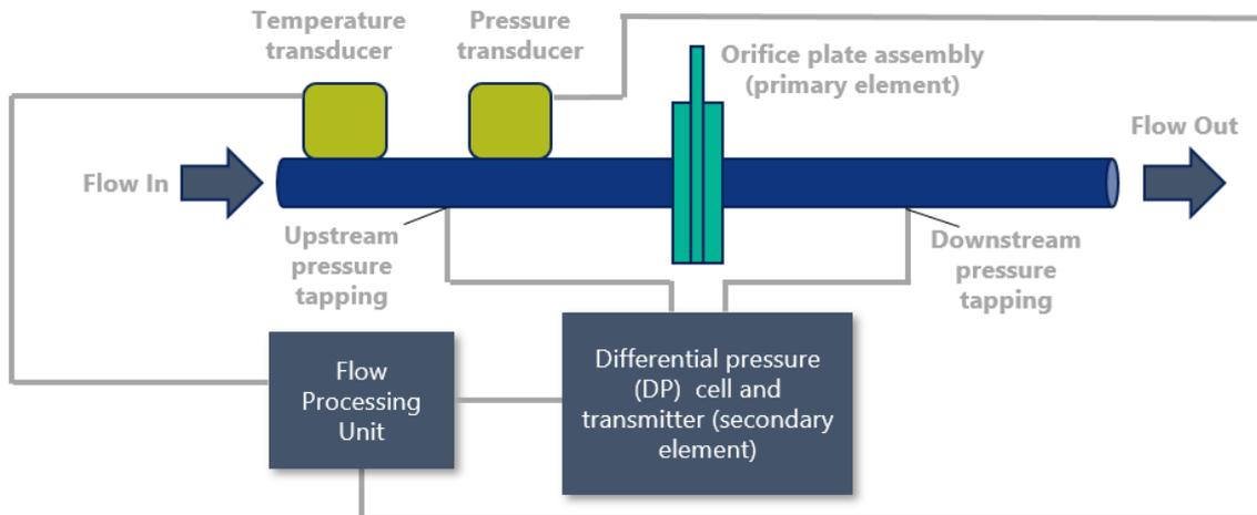
Larger sites use a supervisory control and data acquisition (SCADA) system where flow rate, temperature and pressure readings are transmitted as pulses and a programming software used to calculate energy in steam.
