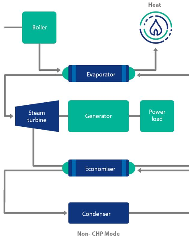
**Figure 3.7: Illustration of an Organic Rankine Cycle (ORC) system operating in a non-CHP mode**
