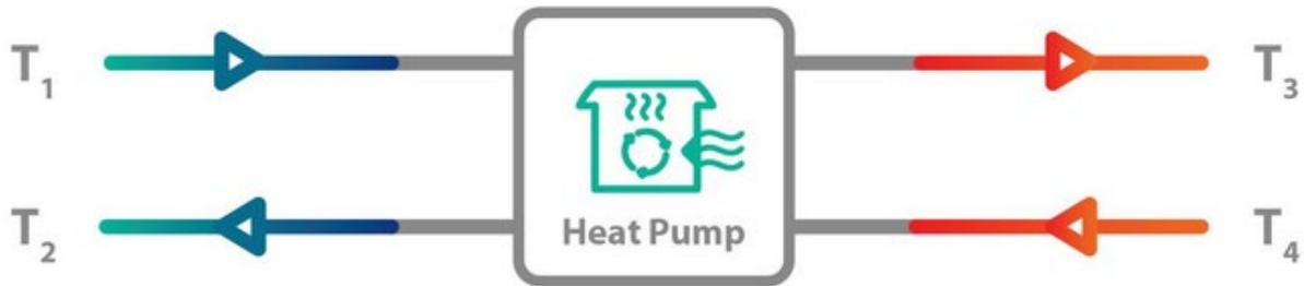
The heat pump system performance depends on the four temperatures shown in Figure 1 above: the flow and return temperature on the heat source ( $T_1$ ,  $T_2$ ), and the flow and return temperature on the heat distribution system ( $T_3$ ,  $T_4$ ). If these temperatures stay within the range required, the heat pump is likely to achieve a seasonal performance factor (SPF), be reliable and require very little maintenance.
