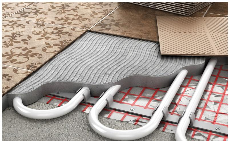
Figure 11: Cutaway of an underfloor heating system
