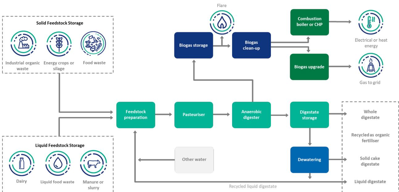
As well as the main anaerobic digester, an AD facility may include some of the components shown in *Table 1*. The equipment indicated in *Table 1* is explained further in the Technology Guide, Section 4.
