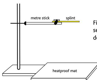
Figure 3: Experimental setup for Fire Clouds demonstration
