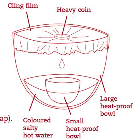
The water collected in the smaller bowl should be clear and not salty. You have distilled pure water from the salty coloured water in the bigger bowl. The water vapour from the boiling salty water rises up to the plastic cover, it cools, condenses and forms water droplets, which run into the smaller bowl. This process is called distillation.
