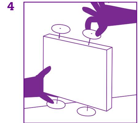
Fix two of the circles to one of the long sides of the polystyrene using pins. Turn the buggy over and fix two wheels on the other long side. Don't push the pins too far into the polystyrene as the wheels may not turn easily: you may need to have a small bead between the wheel and buggy.
