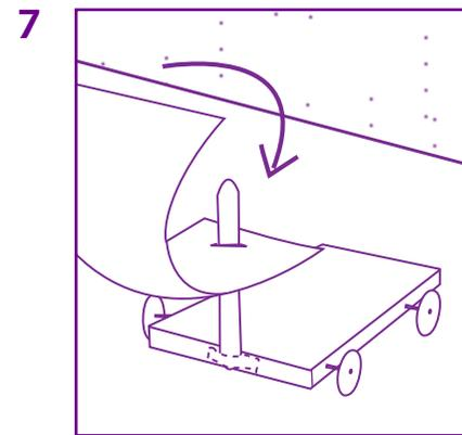
Tape the lolly stick to the front of the buggy. Slide the paper onto the stick by using the small holes made in the paper.
