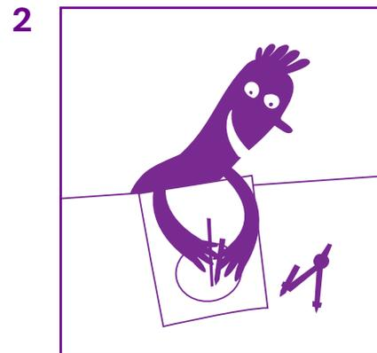
Put a rod or pencil on the centre point made by the compass and draw around this rod/pencil.
