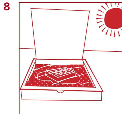
Place the box in direct sunlight with the reflector facing the sun and try melting chocolate in your oven (put it on a plate so you don't make a mess).
