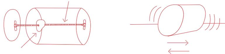
1. Pierce a small hole in the lid and bottom of the can. Make sure the holes are in the centre.
