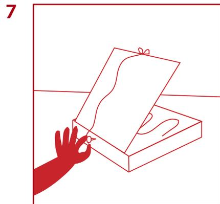
Cut a piece of string and tape one end to the top of the flap. Push a small nail into the back of the box and wrap the string around the nail to keep the flap open.
