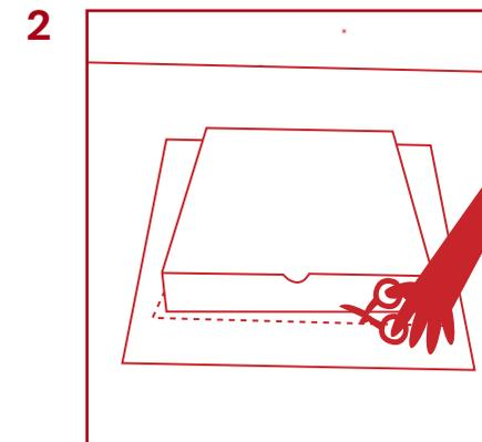
2 Put the box on the plastic and draw the outline of the box on the plastic with the marker. Cut the plastic about 1.25cm inside the mark.
