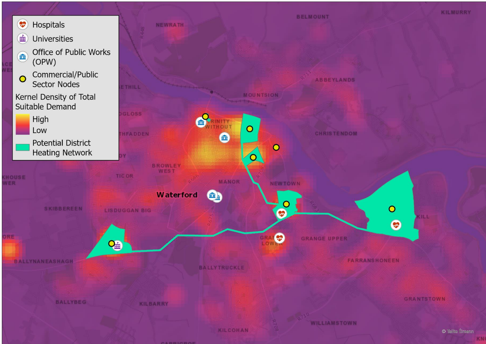
Figure 11: A potential district heating network for Waterford City (Census Divisions suitable for district heating areas manually joined by roads).
