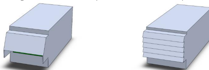
Figure 1 CAD model of an AHU fitted with a (a) single orifice rainhood (Inlet 1) (b) louvre rainhood (Inlet 2) [2].
