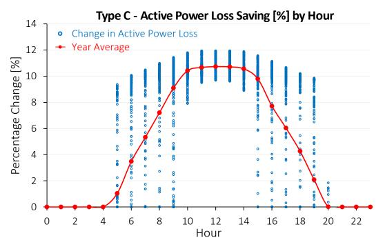
FIGURE 7: TYPE C 10 MW PV INSTALLATION - ACTIVE POWER LOSS REDUCTION ON LINE 0102C BY HOUR
