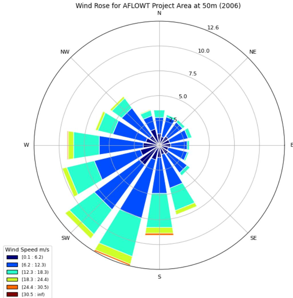
**Figure 7-4: Wind Rise showing wind speed and direction collected at a height of 50m over the year 2006.**
