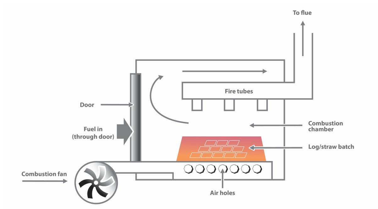
Figure 3.8: 500 kW straw boiler
