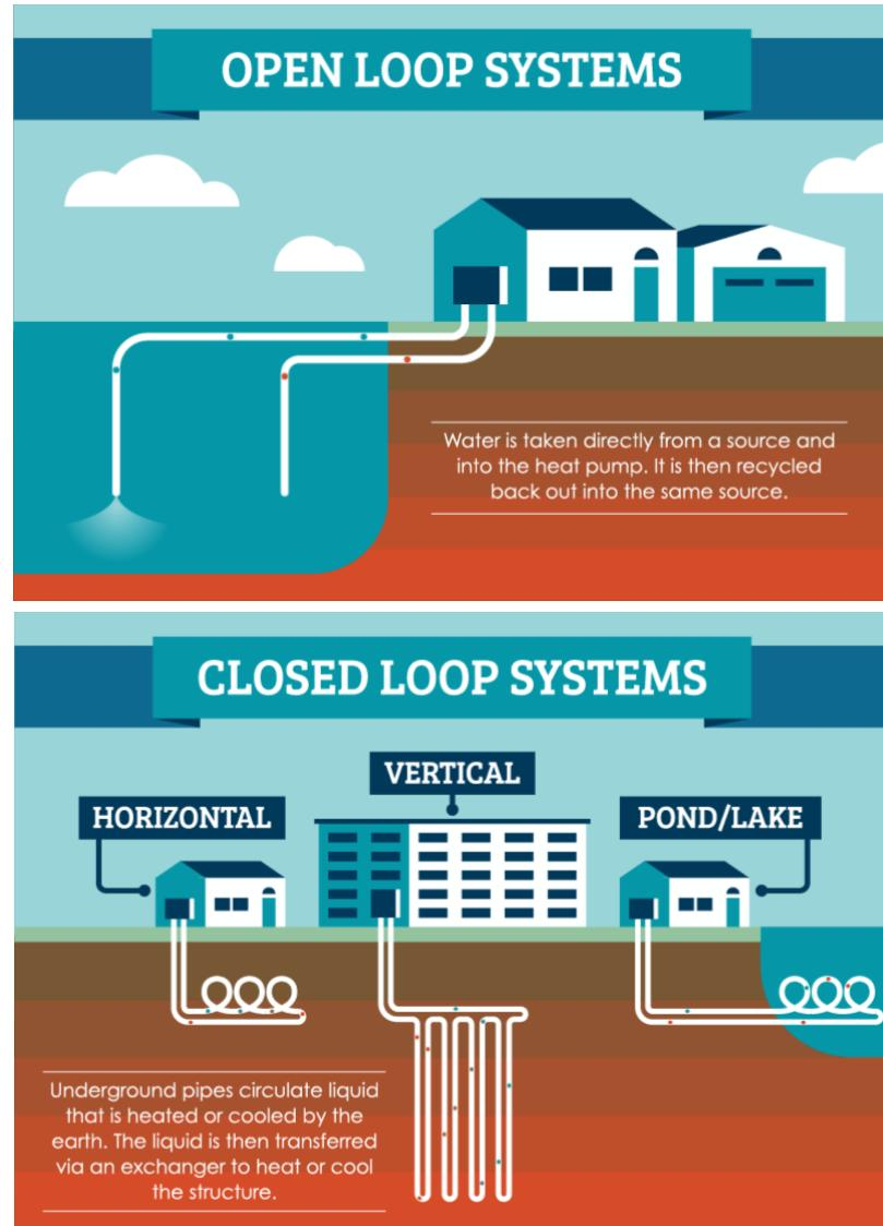
Figure 2: Schematic representation of open loop/closed loop systems
