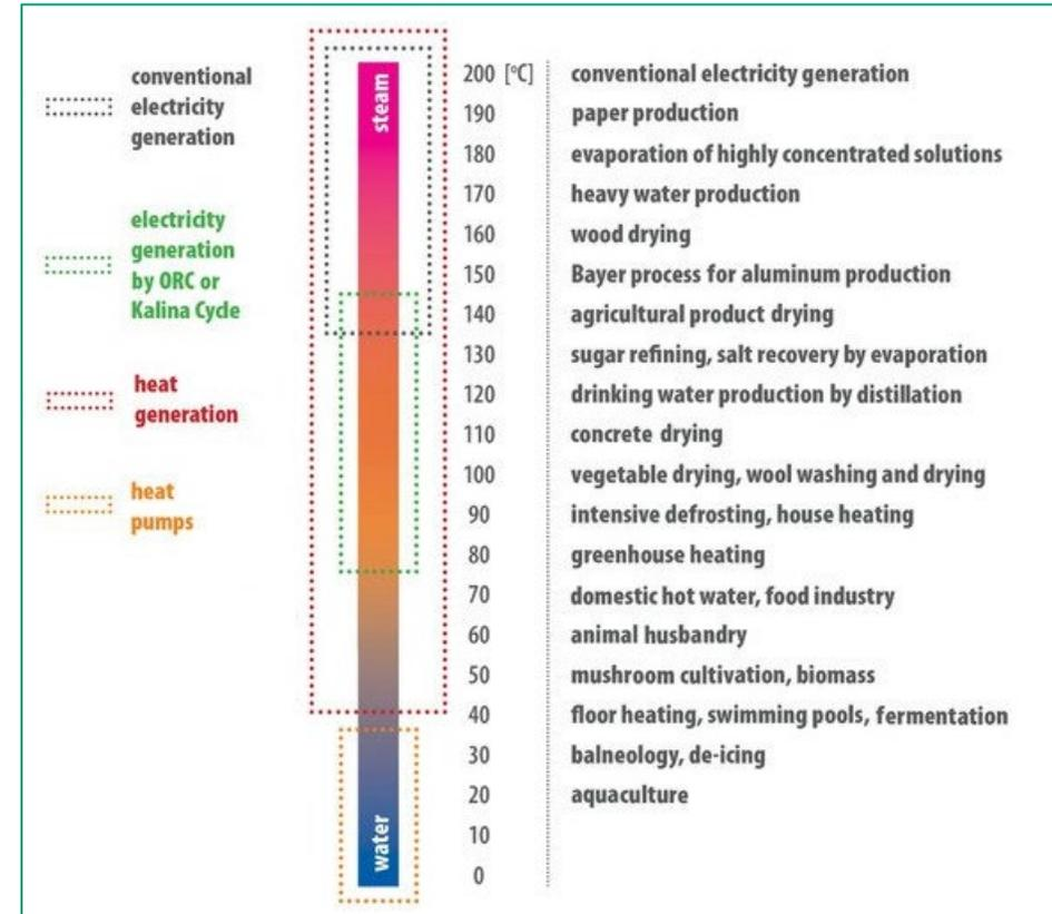
Figure 1: Possible geothermal applications by temperature range and associated technologies.
