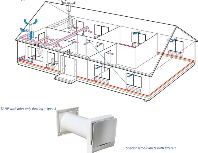
2. EAHP units that provide space and water heating with both supply and exhaust inlet air ducts
