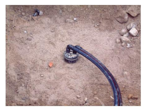
Neoprene borehole sealing cap
