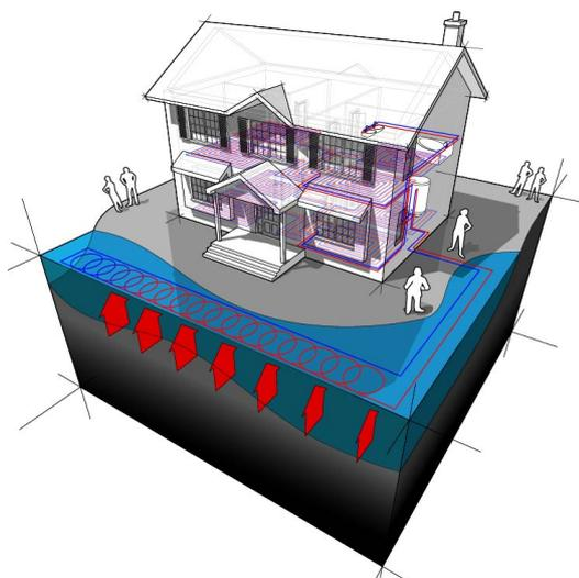
Figure 15: Closed loop surface water-source system
