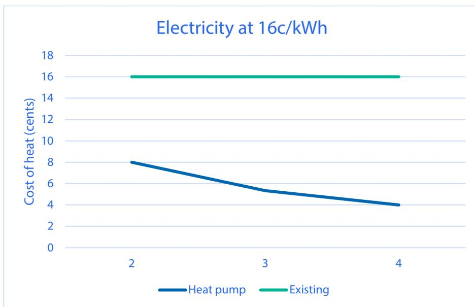
**Figure 4: Cost of heat from a heat pump compared to oil heating (example only)**
