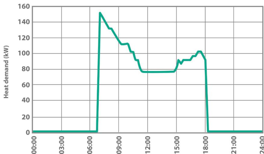
The peak heat demand can be extrapolated from the capacity of existing heat sources (for example, a gas boiler). However, this is often highly inaccurate. The peak heat load may not have been established accurately, and the boiler may have been oversized. Also, the peak heat demand could have changed since the boiler was installed.
