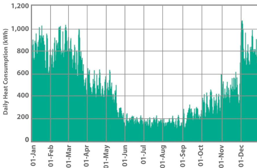
There are several methods for estimating the total heating requirement of a building, each with different levels of complexity and accuracy. Whichever method is used, a calculation of the total heat used by a building in a year is always a simulation based on the expected use of the building. The real heat usage fluctuates based on weather and operating patterns.
