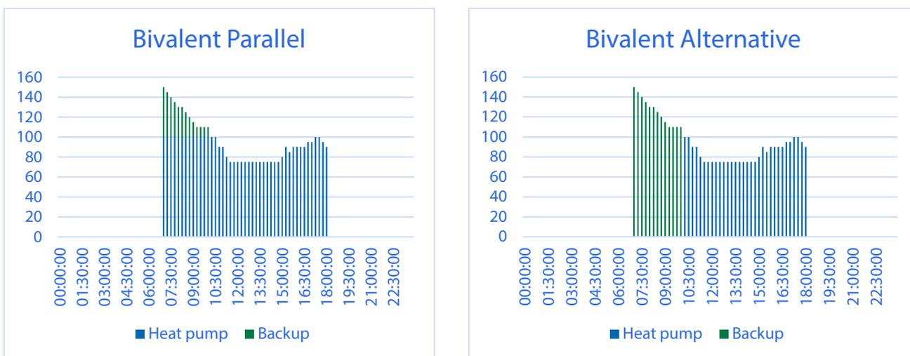
Bivalent parallel operating mode should result in the heat pump providing a greater proportion of the overall demand (see Figure 16). However, parallel operation is not always possible.
