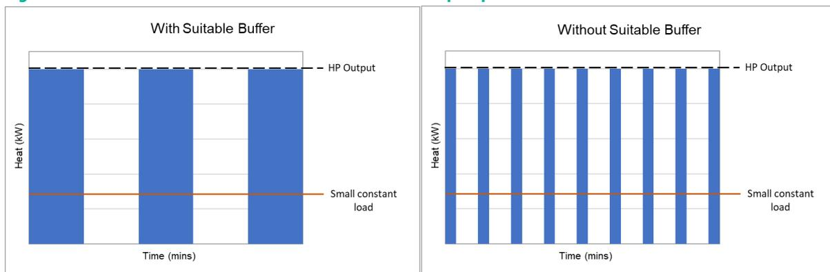
Using a thermal store also gives more control over heat pump operation. Heat is stored for later use. This means that system costs are lower, because the heat pump can operate during periods of cheaper 'off-peak' electricity.
