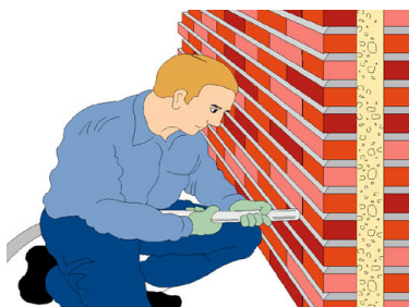
2. Cavity Wall Insulation
