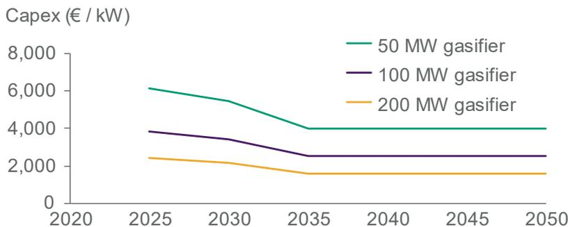
The costs shown in Figure 26 for biomass gasification are based on two academic papers [31] [32]. The efficiency of biomass gasification shown in Figure 27 was developed using the same sources. The cost assumptions for the biomethane transport options considered are presented in Table 10 below.
