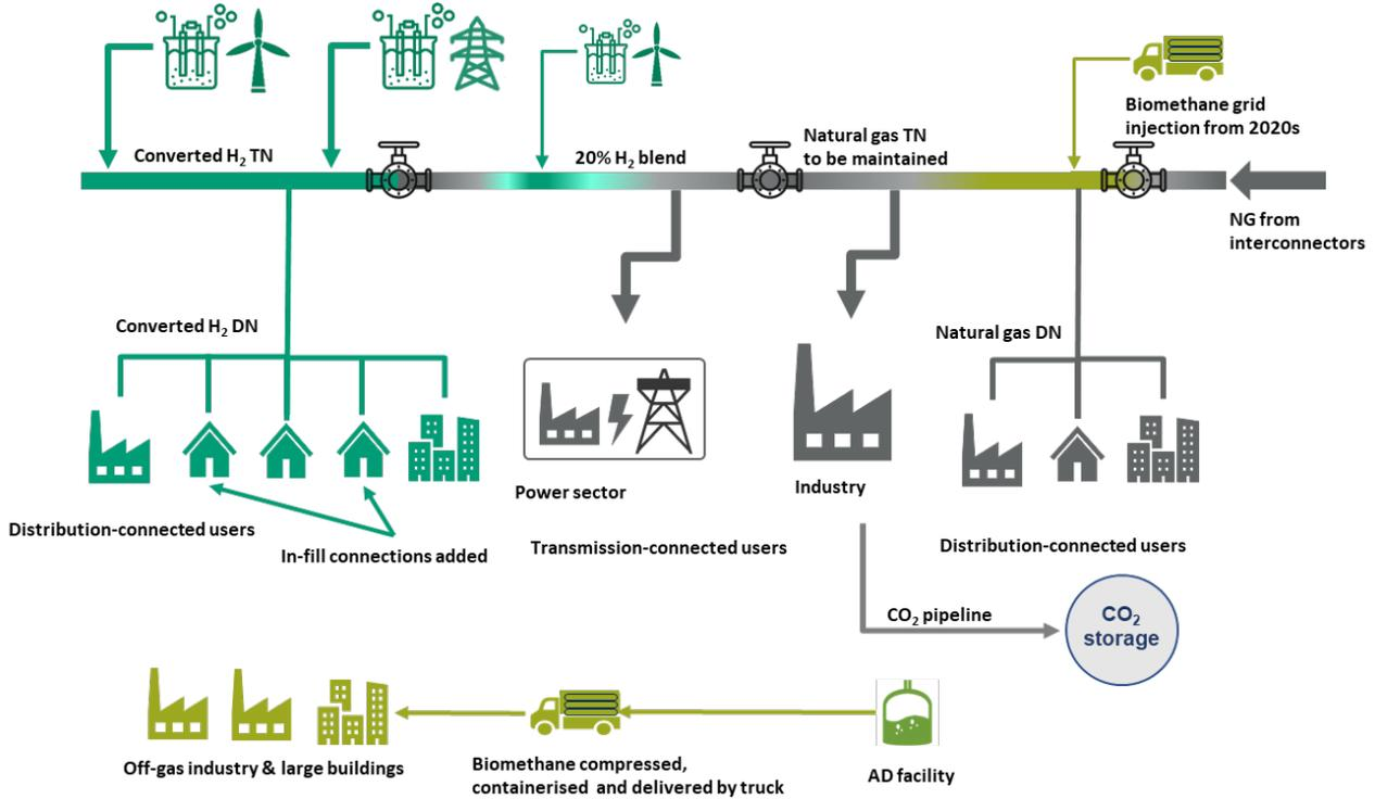
**Figure 17: Potential sequence of the piecemeal network conversion**
