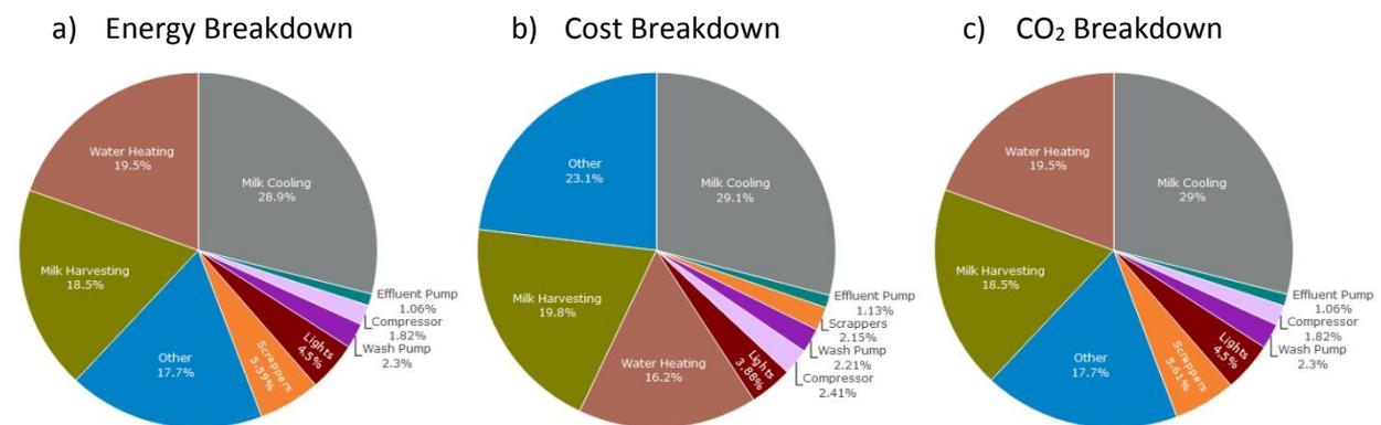
Figure 4: Pie charts presenting energy consumption (a), cost (b) and CO<sub>2</sub> emissions (c) breakdowns (downloaded from DSSSED tool using default input parameters)
