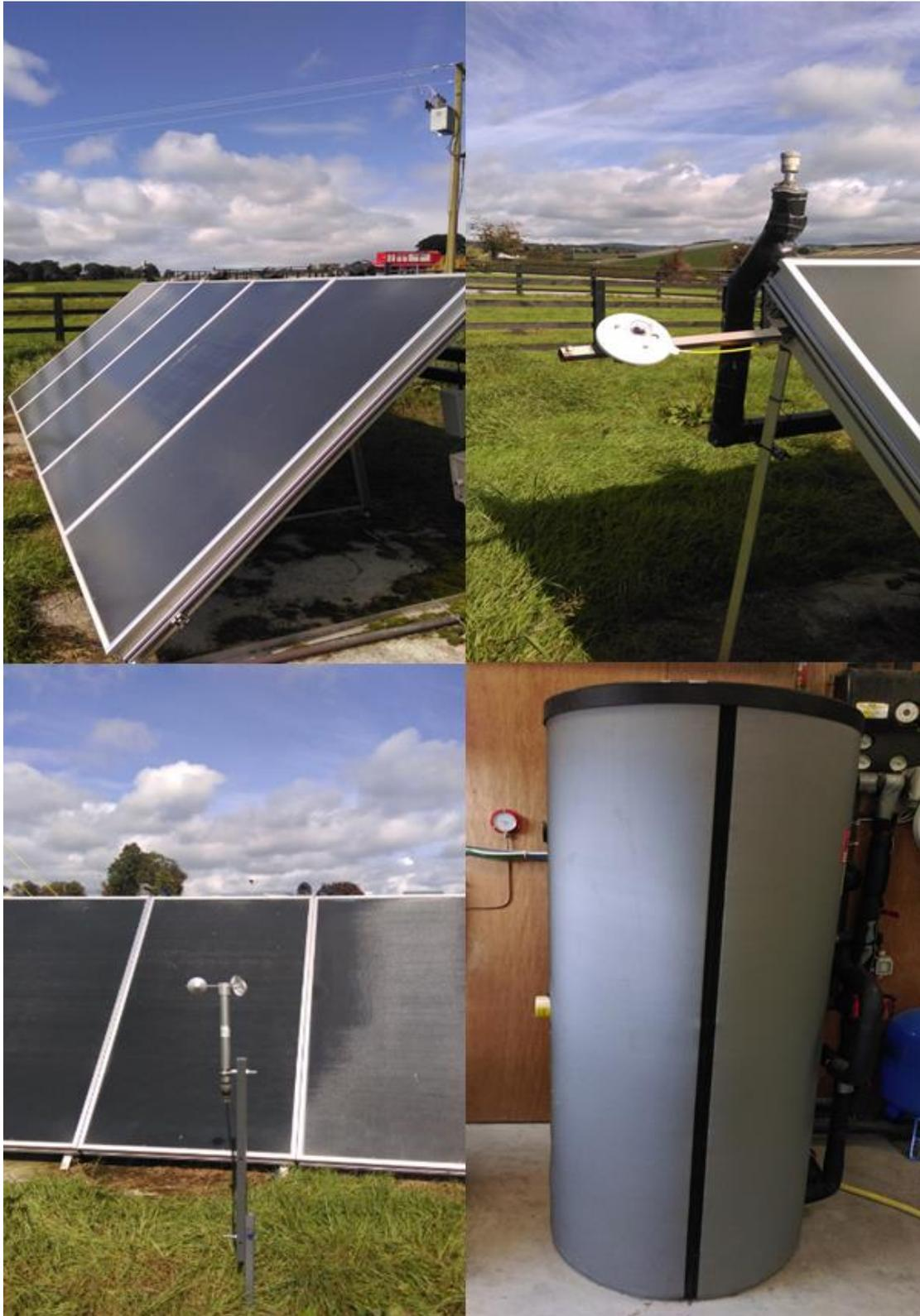
Figure 9: Equipment used for solar water heating experiments, clockwise from top left: Solar panel array; Pyranometer to measure irradiance; Water tank to which heat was transferred; Anemometer to measure wind speed.
