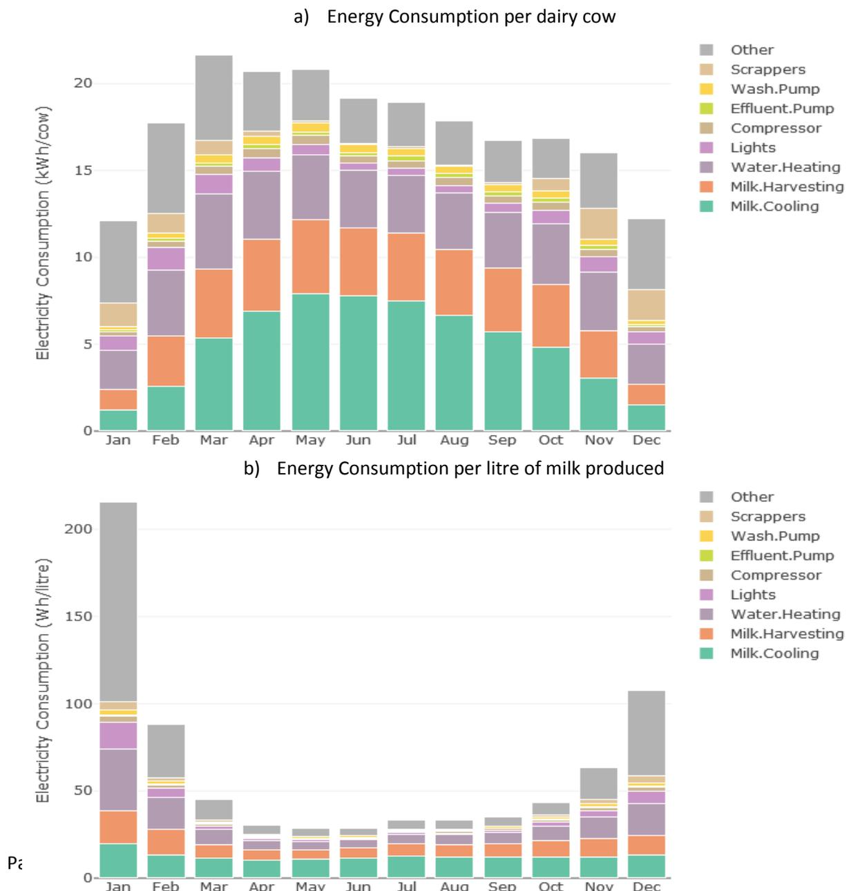
Figure 5: Mean monthly energy consumption per dairy cow (a) and per litre of milk produced (b) for each energy consuming process
