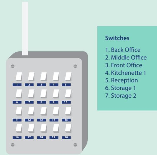
Figure 11: Open plan switch bank with area switches and master off switch
