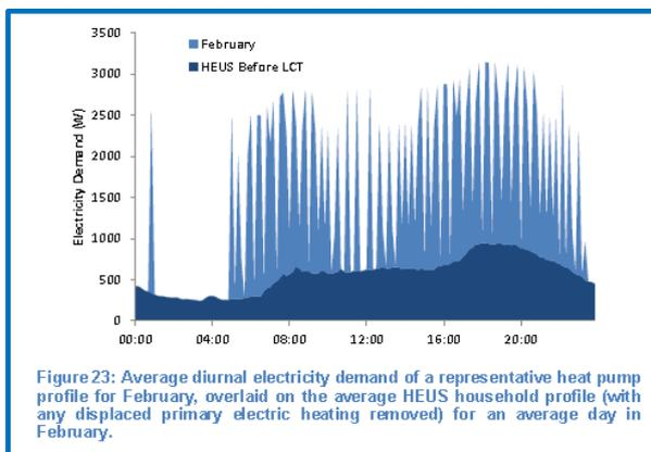
Figure 23: Average diurnal electricity demand of a representative heat pump profile for February, overlaid on the average HEUS household profile (with any displaced primary electric heating removed) for an average day in February.
