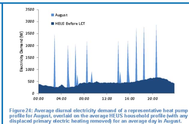
Figure 24: Average diurnal electricity demand of a representative heat pump profile for August, overlaid on the average HEUS household profile (with any displaced primary electric heating removed) for an average day in August.
