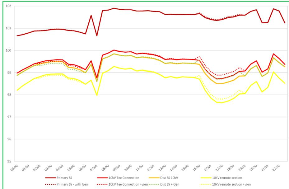
**FIGURE 14 – WINTER MAXIMUM VOLTAGE DIURNAL PROFILE ON THE MV FEEDER**
