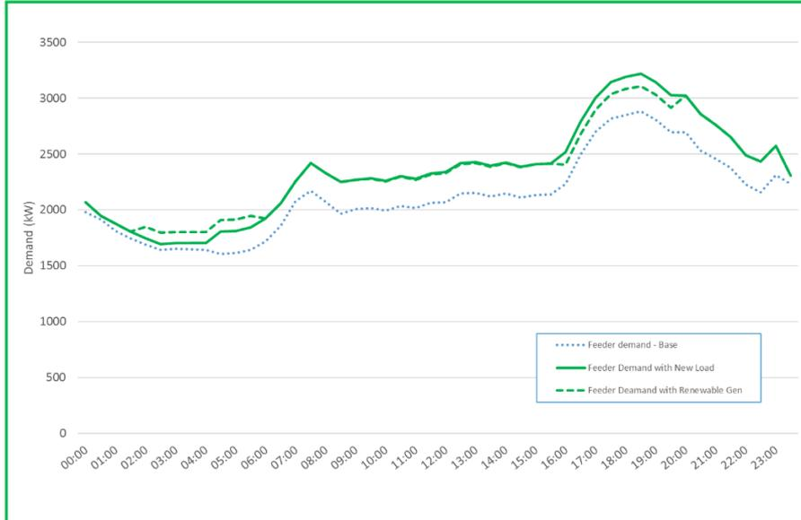
**FIGURE 8 – WINTER DIURNAL DEMAND PROFILE AT THE MV FEEDER CIRCUIT**
