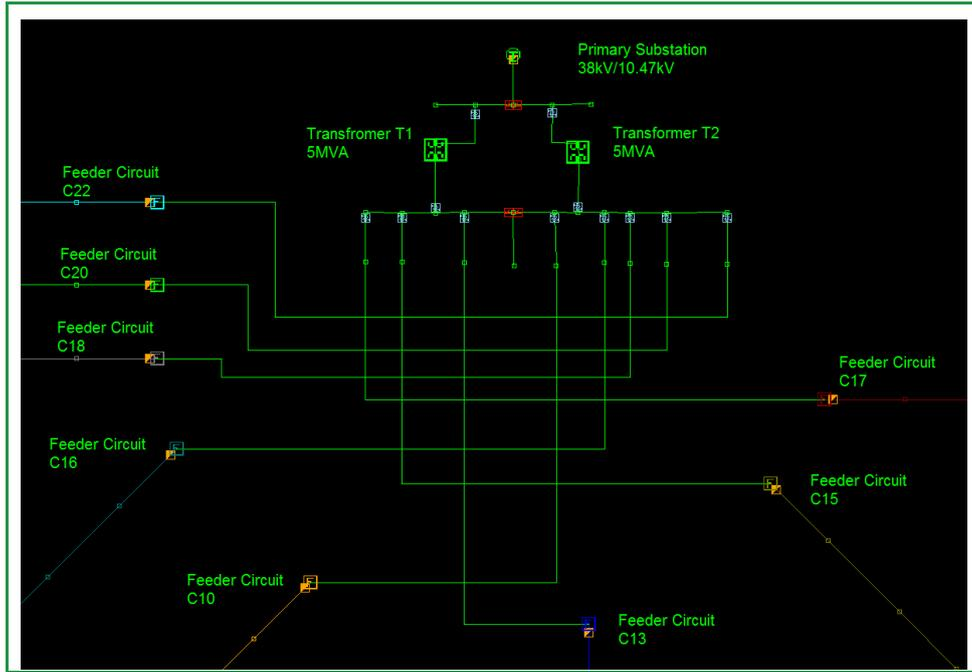
FIGURE 20 – PRIMARY SUBSTATION SINGLE LINE DIAGRAM
