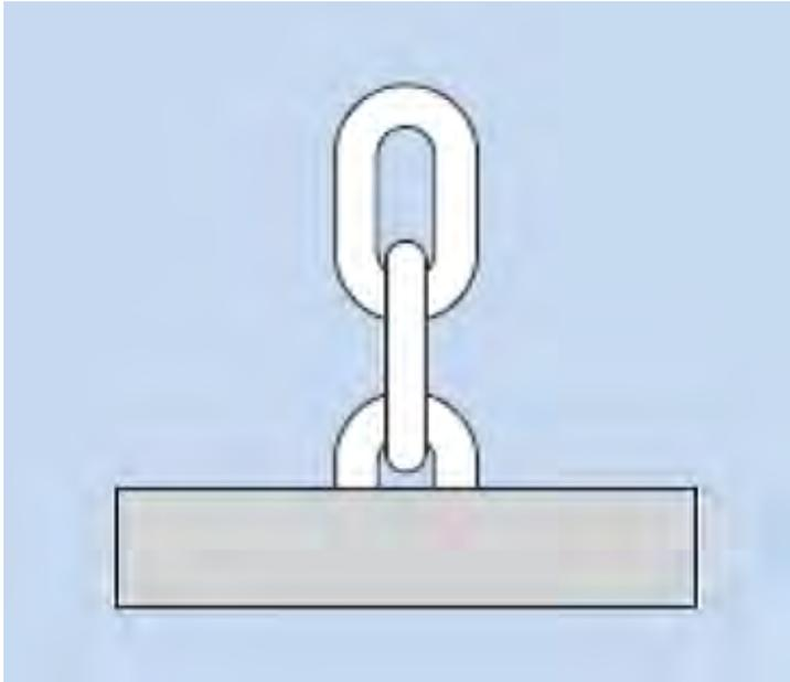
**Figure 4-30: Sketch of typical gravitation anchor**
