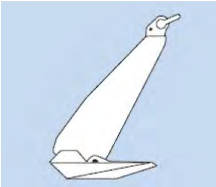
**Figure 4-31: Sketch of a drag embedment anchor**
