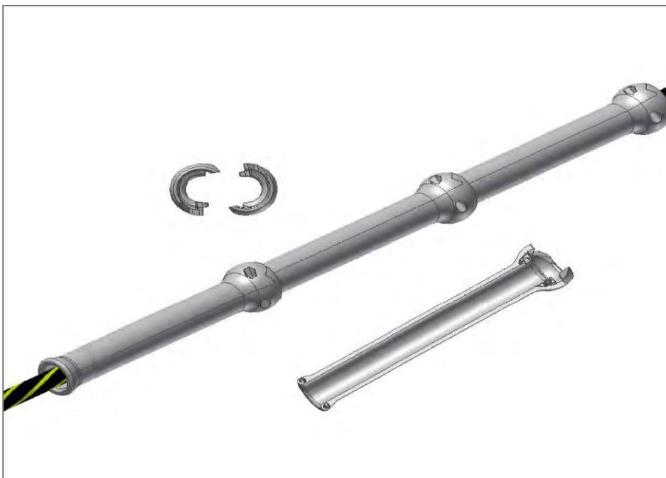
**Figure 4-8: Split shell cable protection**
