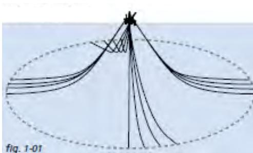
**Figure 4-28: Example of catenary mooring system**
