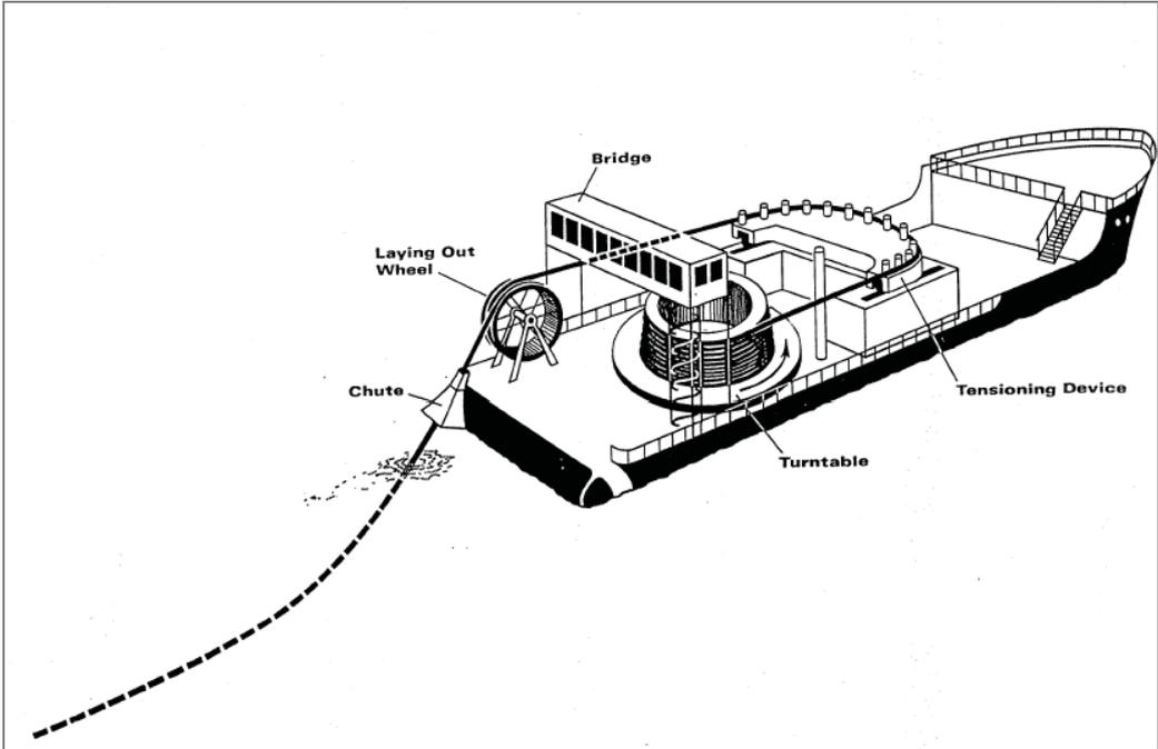
Figure 4-24: Sketch of typical cable lay vessel
