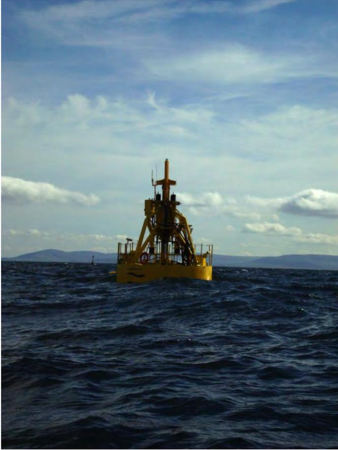
**Figure 4-15: Quarter scale Wavebob WAB-PA device**
