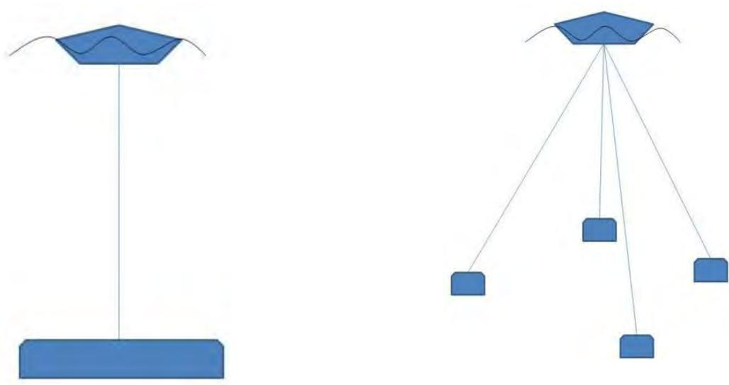
**Figure 4-27: Typical single and spread mooring system**
