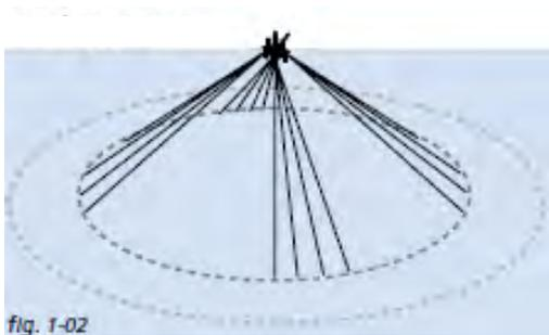
**Figure 4-29: Example of taut leg mooring system**
