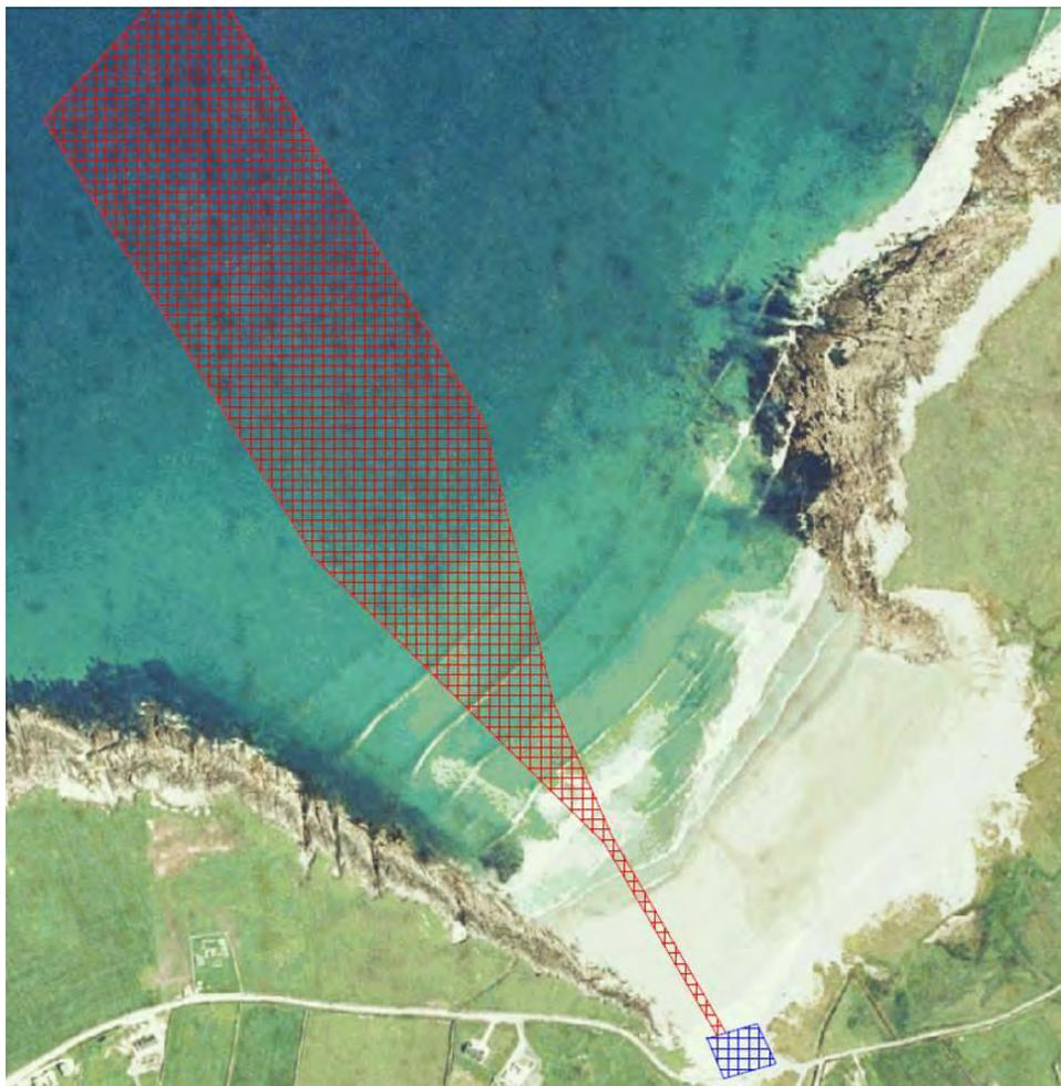
**Figure 4-21: Proposed route of cable trench across Belderra Strand**
