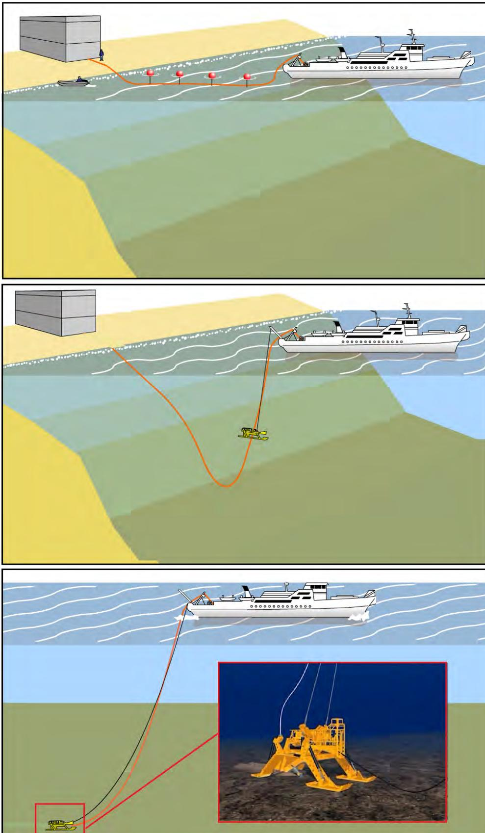
**Figure 4-9: Schematic of typical off-shore cable laying operation**
