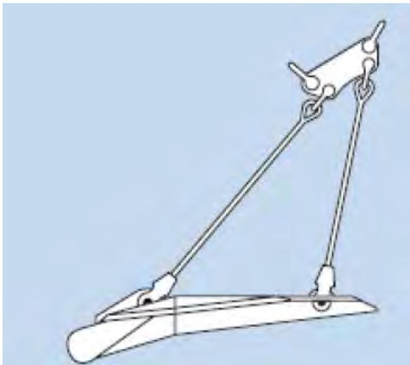
**Figure 4-32: Sketch of a vertical load anchor**
