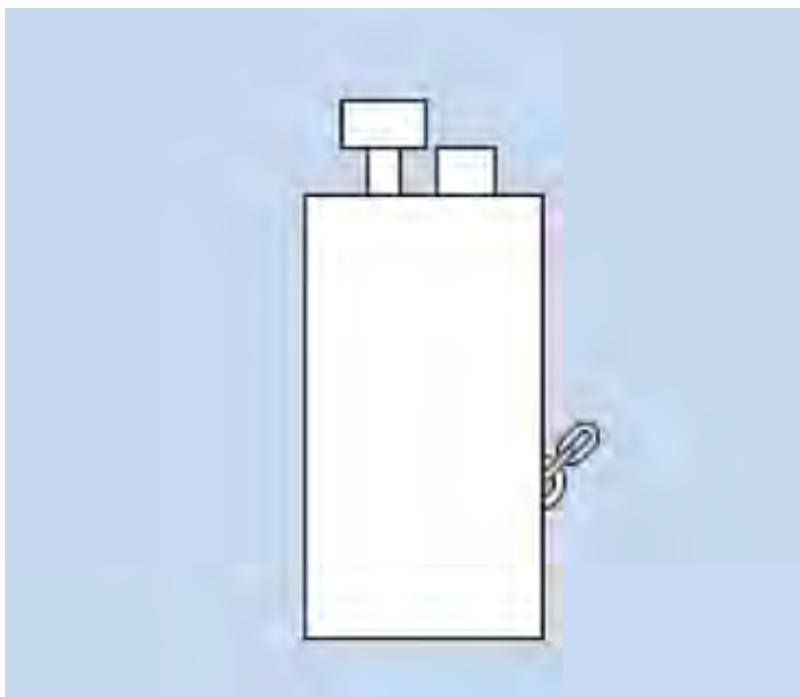
**Figure 4-33: Sketch of a suction bucket anchor**
