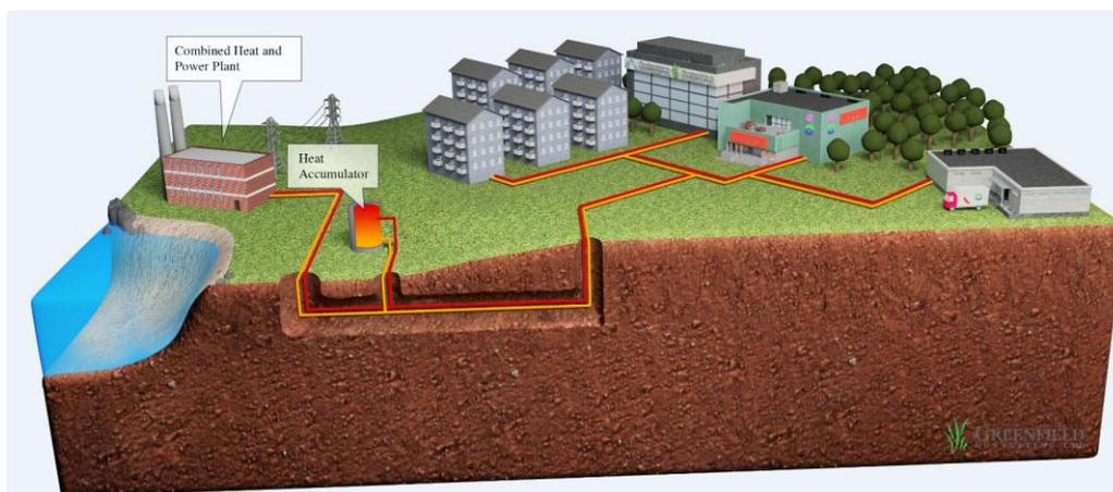
Figure 6: Illustration of a heat network<sup>8</sup>
