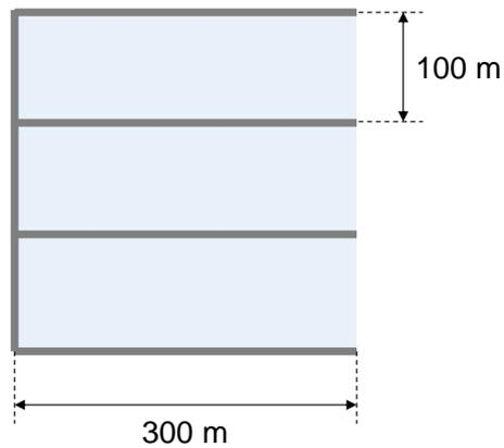
**Figure 22: Illustration of a distribution network route (grey lines) supplying a square 9 hectare (300m x 300m) area (blue fill), assuming a block size of 100m. The distribution network length is 1.5 km.**
