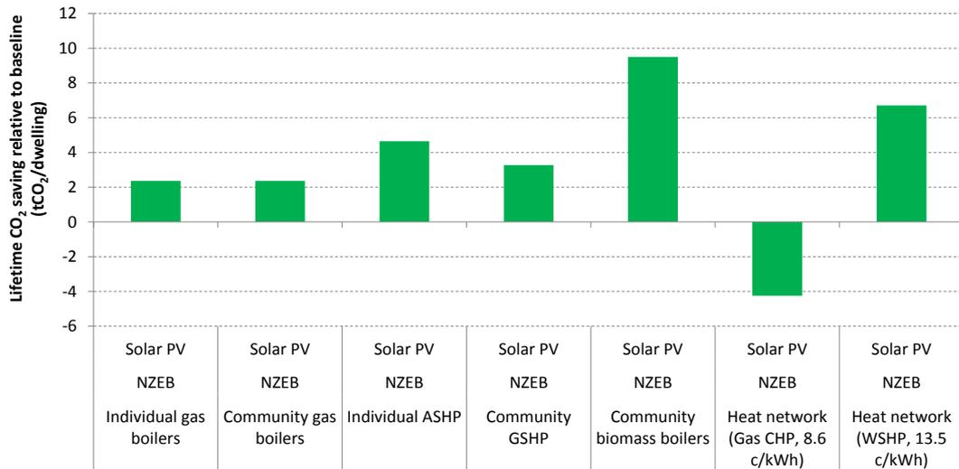
Figure 48: Lifetime CO<sub>2</sub> savings: variation with different heating systems (mid-floor apartment)
