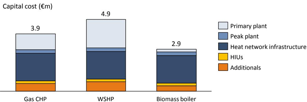
Figure 27: Capital cost for “Fonthill only (All)” scheme, comparison of Gas CHP, WSHP and Biomass boiler heat supply options in the emerging preferred scenario (note: ‘Additional’s’ represents a 15% contingency)
