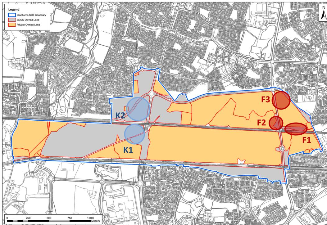
**Figure 21: Energy centre location options for heat network schemes based at Fonhill (shown in red) and Kishoge (shown in blue).**
