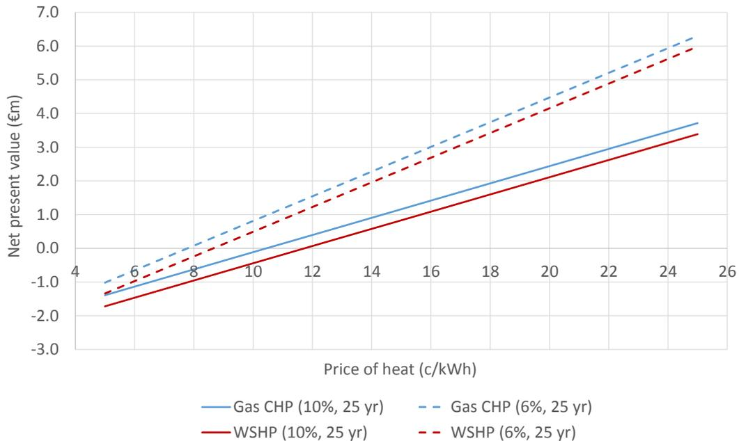
**Figure 29: Net present value (25 years) as a function of price of heat for the “Kishoge only (All)” scheme, schemes based on Gas CHP and WSHP with RHI (Emerging preferred scenario)**
