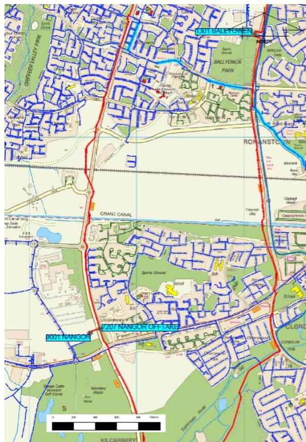
Figure 20: Gas infrastructure map showing high pressure gas transmission pipes (shown in red) in the vicinity of the SDZ [Source: Gas Networks Ireland via SDCC]
