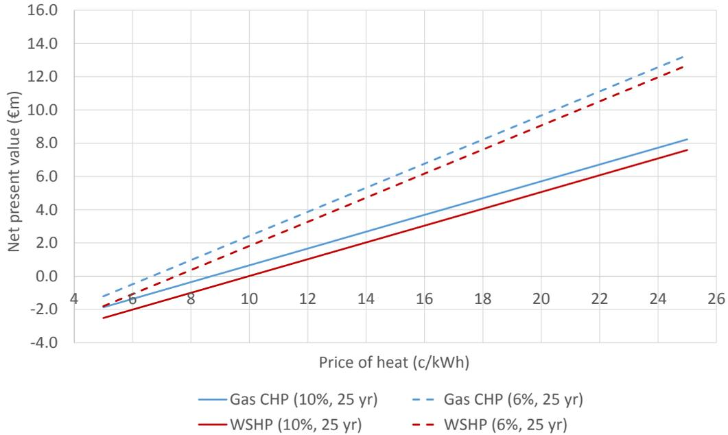
**Figure 28: Net present value (25 years) as a function of price of heat for the “Fonhill only (All)” scheme, schemes based on Gas CHP and WSHP with RHI (Emerging preferred scenario)**
