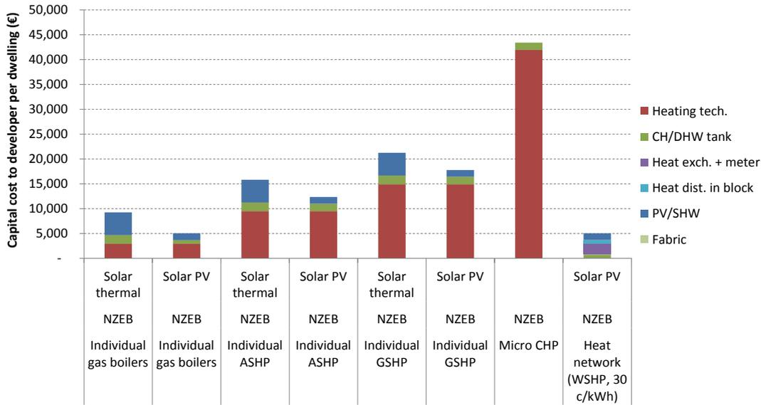
Figure 42: Capital cost to developer: variation with different heating systems (semi-detached house)
