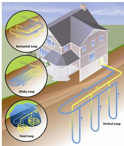
Figure 55: Options for ground source heat pump heat collectors<sup>38</sup>
