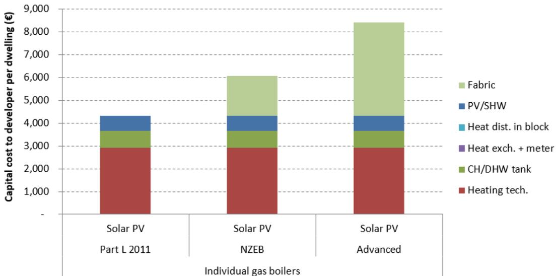
Figure 34: Capital costs to developer: variation with level of fabric energy efficiency for a mid-floor apartment (see footnote for explanation of the terms in the legend<sup>31</sup>)
