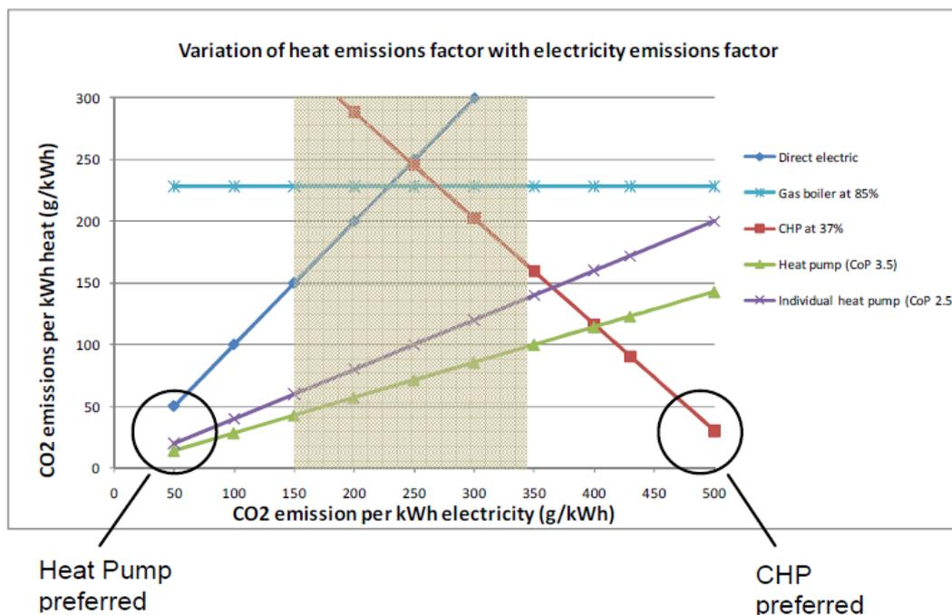
**Figure 8: Variation of the CO<sub>2</sub> intensity of heat generated for gas CHP, heat pumps and conventional heating technologies as the grid carbon intensity varies<sup>15</sup>.**
