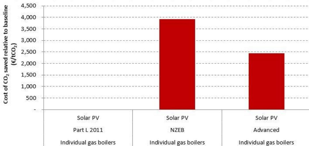
Figure 39: Cost of CO<sub>2</sub> savings achievable through different levels of fabric efficiency (semi-detached house with solar PV)
