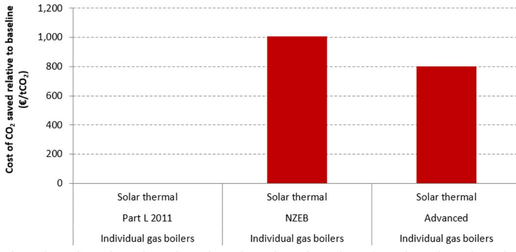
**Figure 40: Cost of CO<sub>2</sub> savings achievable through different levels of fabric efficiency (semi-detached house with solar thermal)**
