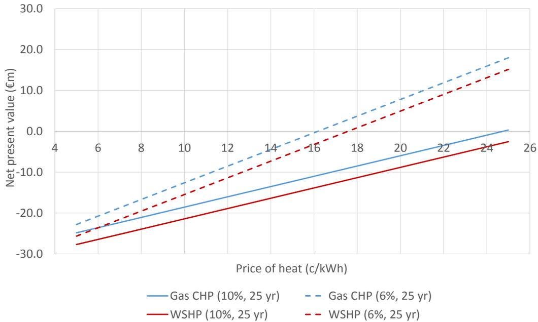
**Figure 30: Net present value (25 years) as a function of price of heat for the “Fonthill and Kishoge” scheme, schemes based on Gas CHP and WSHP with RHI (Emerging preferred scenario)**
