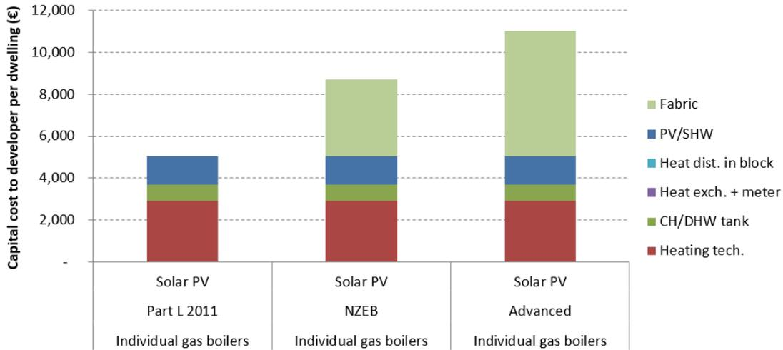
**Figure 35: Capital costs to developer: variation with level of fabric energy efficiency for a semi-detached house**
