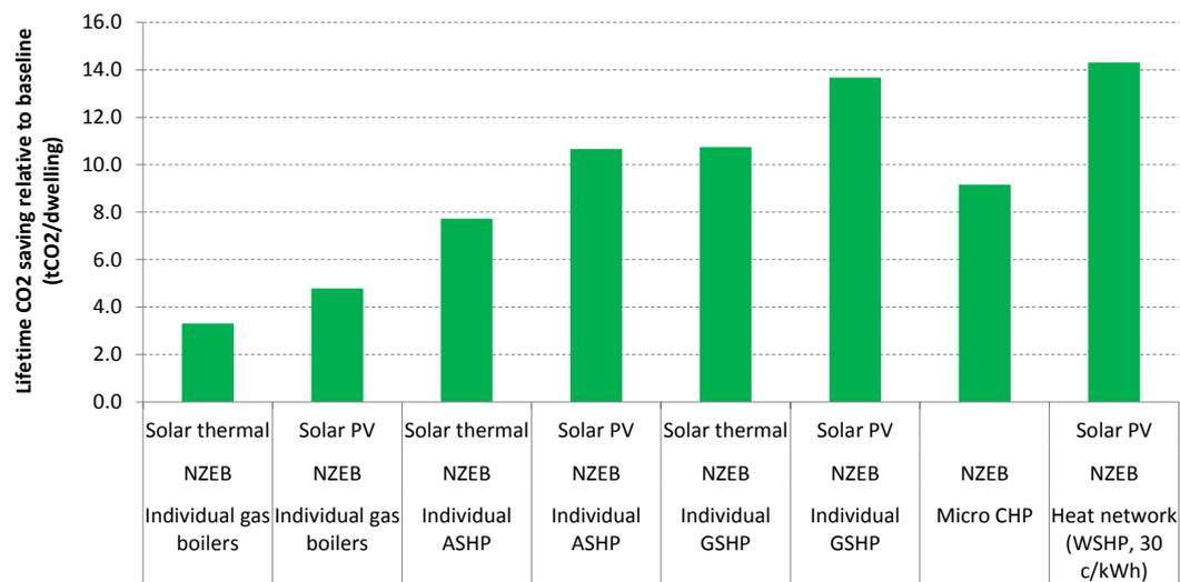
Figure 49: Lifetime CO<sub>2</sub> savings: variation with different heating systems (semi-detached house)
