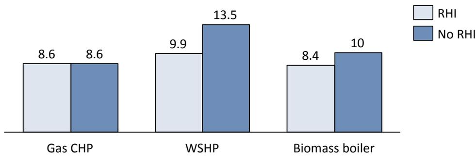
Figure 26: Price of heat required to achieve 10% rate of return for “Fonthill only (All)” scheme, comparison of Gas CHP, WSHP and Biomass boiler heat supply options (Emerging preferred scenario)
