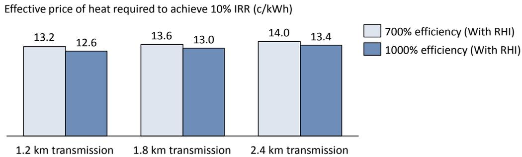
**Figure 32: Price of heat required to achieve 10% rate of return for “Kishoge only (All)” scheme supplied by waste heat from Grange Castle with WSHP, for various transmission pipe lengths and WSHP efficiencies (Emerging preferred scenario)**
