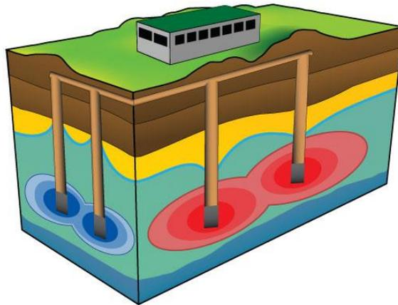
**Figure 11: Schematic of an open-loop system involving abstraction and rejection of aquifer water. Image courtesy of G-Core (2016).**
