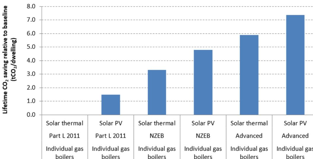
Figure 37: Lifetime CO<sub>2</sub> savings achievable through different levels of fabric efficiency (semi-detached house)
