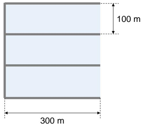
**Figure 22: Illustration of a distribution network route (grey lines) supplying a square 9 hectare (300m x 300m) area (blue fill), assuming a block size of 100m. The distribution network length is 1.5 km.**
