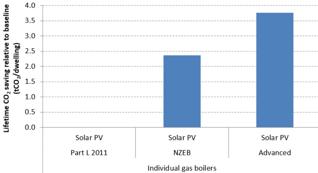
Figure 36: Lifetime CO<sub>2</sub> savings achievable through different levels of fabric efficiency (mid-floor apartment)
