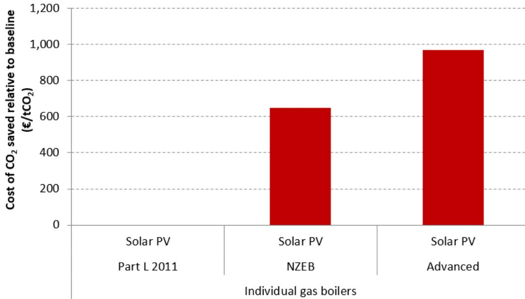
Figure 38: Cost of CO<sub>2</sub> savings achievable through different levels of fabric efficiency (mid-floor apartment with solar PV)
