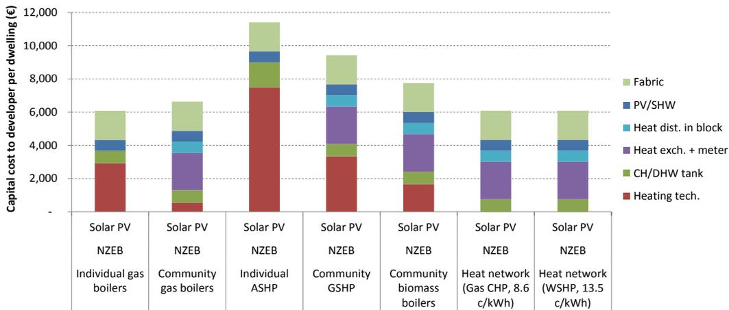
Figure 41: Capital cost to developer: variation with different heating systems (mid-floor apartment)<sup>32</sup>
