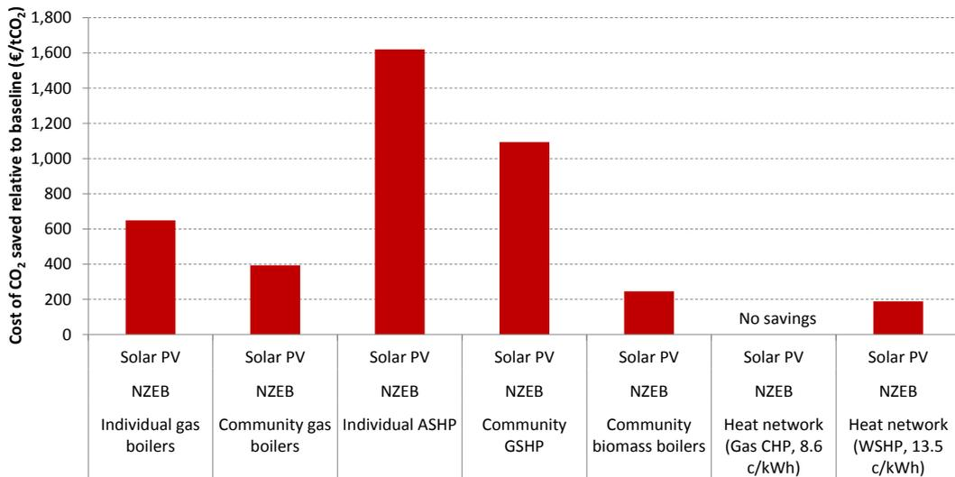
Figure 50: Cost of CO<sub>2</sub> savings: variation with different heating systems (mid-floor apartment)
