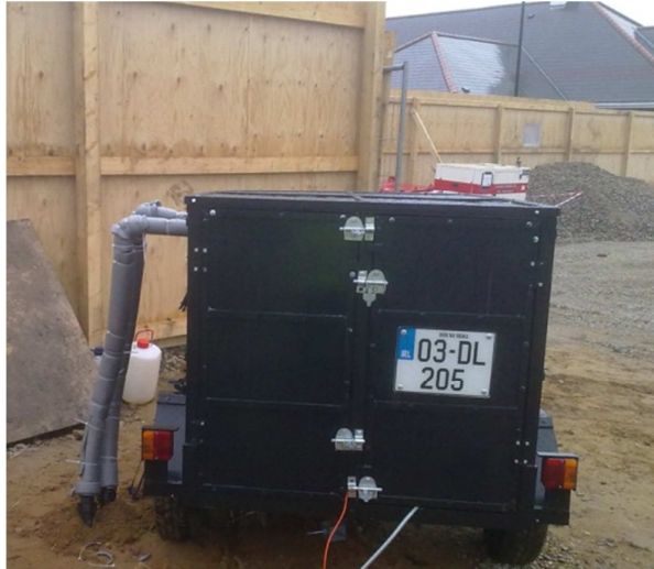
Figure 17: Thermal Response Test rig. Note insulated connections to heat collector at left.
