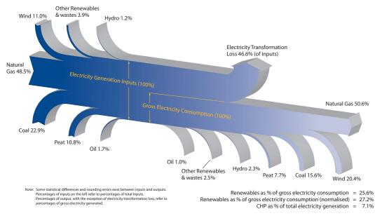
Figure 11: Flow of Energy in Electricity Generation 2016 – Outputs by Fuel
