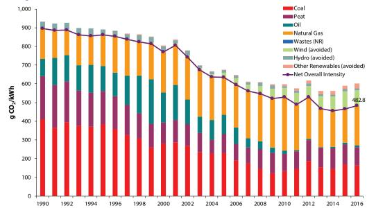
*Figure 13* shows as stacked bars the shares of the various fuels contributing to the overall emissions intensity, as well as the reduction in intensity as a result of emissions avoided by renewable generation from wind, hydro and other renewables. It is important to note that this graph represents the shares of the fuels to the overall intensity and not the intensity of the generation by the individual fuels themselves. The net overall intensity is shown as a line graph in *Figure 13*.
