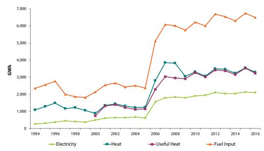
Figure 14: CHP Fuel Input and Thermal/Electricity Output 1994 – 2016
