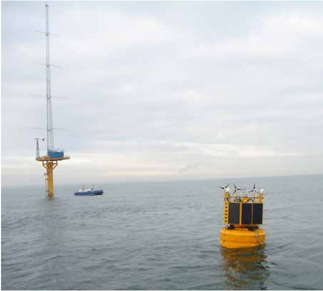
Figure 5. FLiDAR floating lidar system (Source: www.leosphere.com/products/floating/flidar-floating-buoy-lidar )
