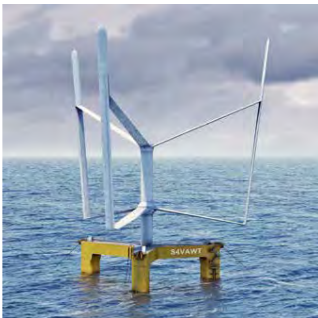
Figure 4. Semi-submersible floater for a large vertical axis turbine being designed by ECN
