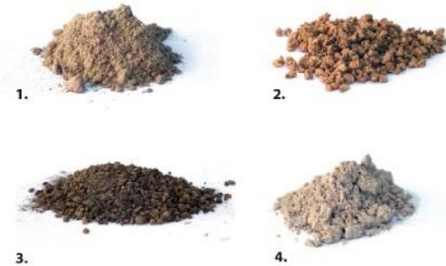
1. Diatomaceous earth / 2. Cork / 3. Clay / 4. Natural hydraulic lime
