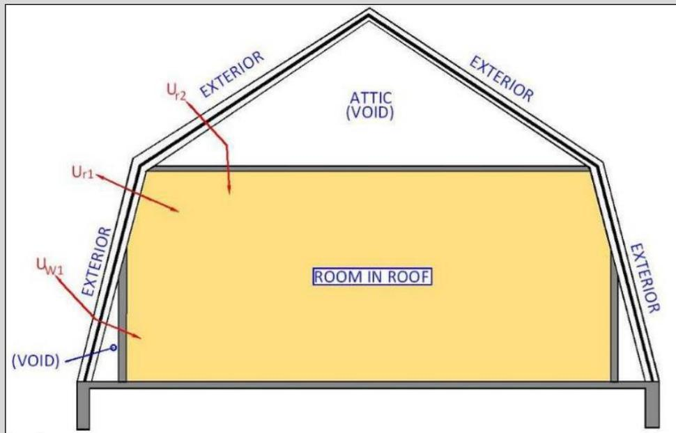
The “connects to” is to exterior as indicated by the red arrows. The construction of the wall or the ceiling with the void includes the airspace as part of the construction. The U-values for these constructions,  $U_{r2}$  and  $U_{w1}$ , are calculated including the void and exterior façade.
