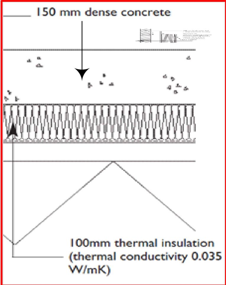
Material thicknesses from as-built drawings.
