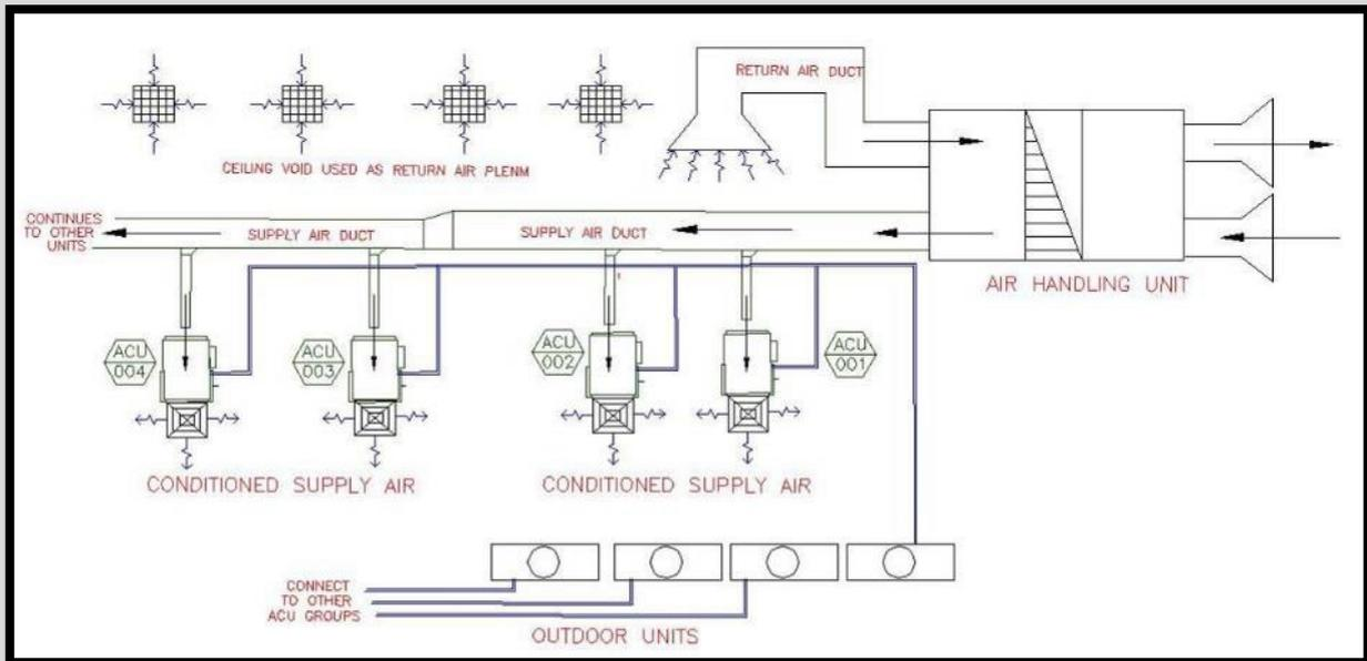
In iSBEMie: Type is a “split or multi-split system”. The heat source is “air source heat pump” (fuel is electricity).
