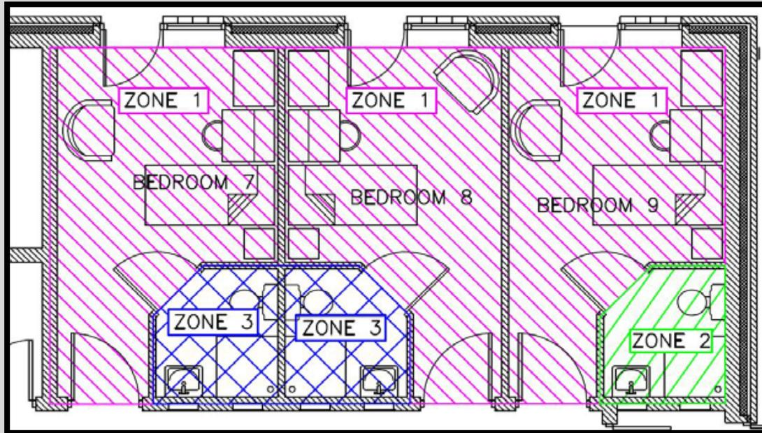
The three bedrooms can be merged into one zone as they are touching (contiguous), have identical HVAC, lighting, activity, and their daylight aspect is also identical. The bathrooms cannot be merged into the bedroom zones as they have a different lighting to the bedrooms. Two bathrooms have been merged as they are contiguous. The third bathroom is not contiguous to another bathroom, so it must be defined as its own zone.
