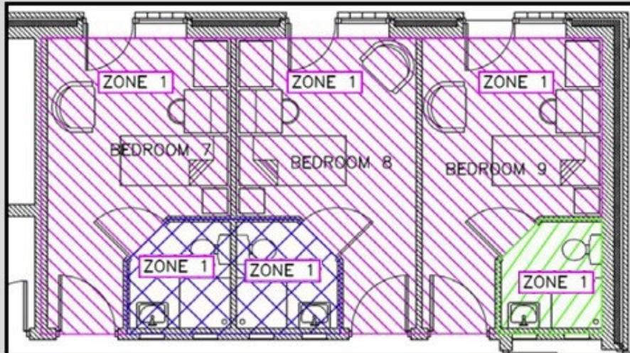
If we were to combine the en-suites and the toilets, one exhaust flow rate would be applied to the combined space. The exhaust flow rates would represent the entire room, so would result in an incorrect result.
