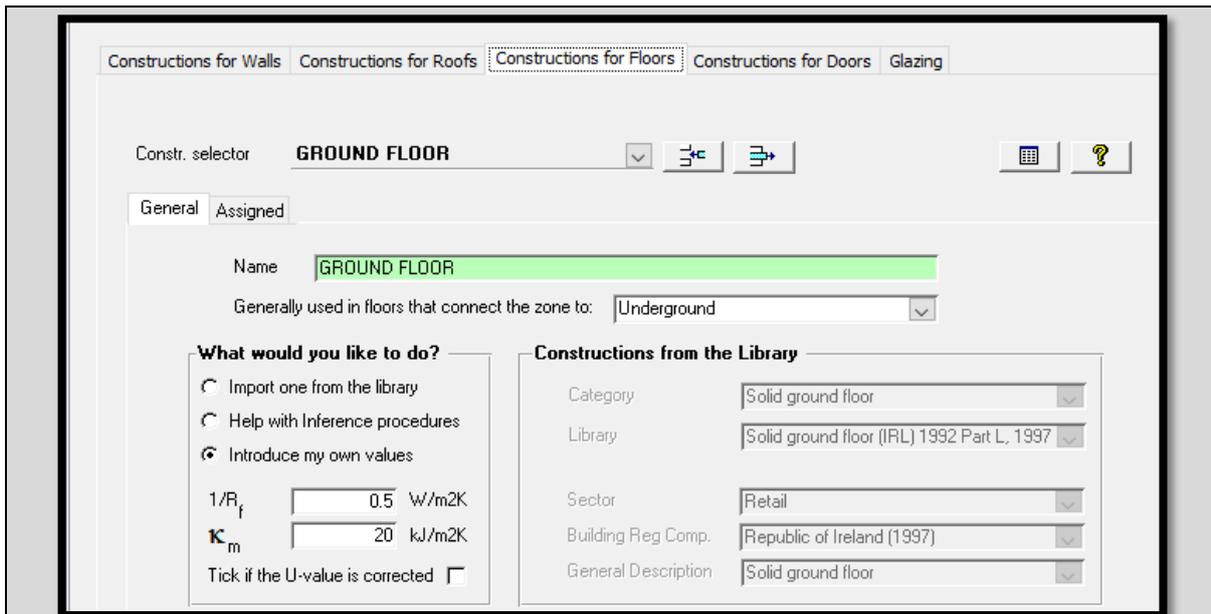
The U-value and  $K_m$  figures are copied to match the values that were obtained in iSBEM Version 3.5.b and appear in the “Introduce my own values section”. However, when the default is selected for the 5.5h version of the iSBEMie software, the U-value changes to 0.45 and the  $K_m$  value also changes. This updated value, shown below, is what an assessor must use.
