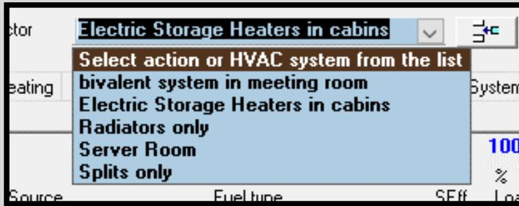
The left screenshot shows that this example building has multiple HVAC systems. **Be careful to select the correct system to make bi-valent.**
