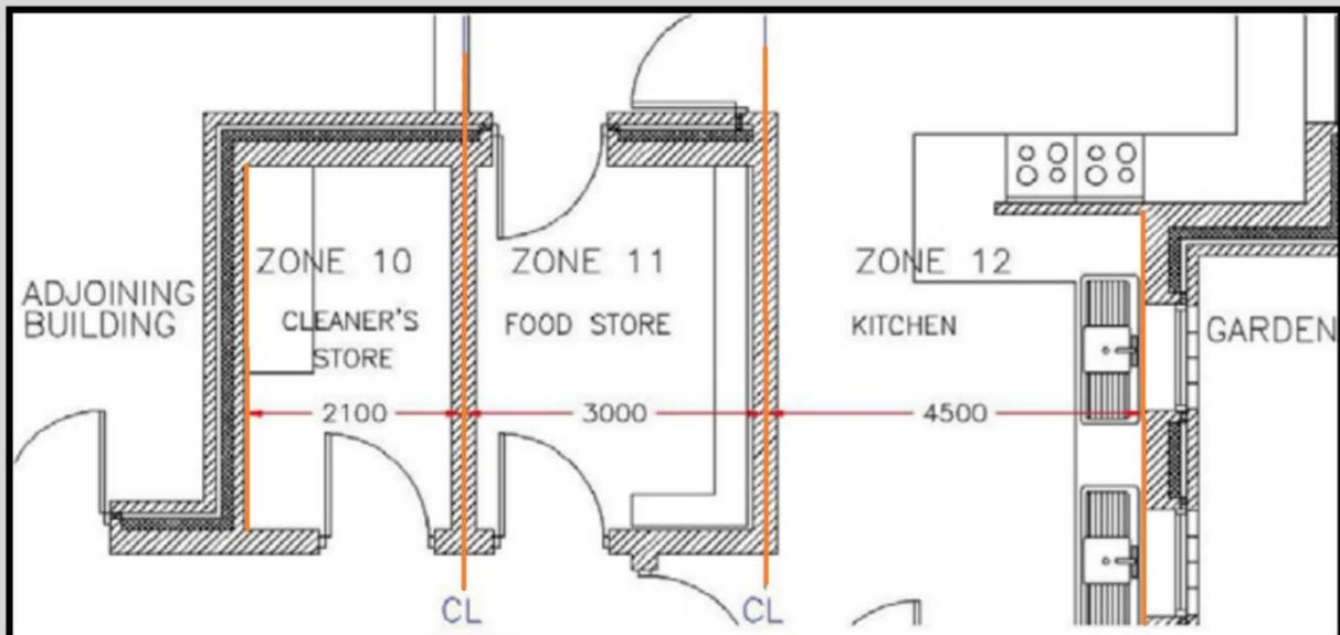
External or party walls bounding adjoining buildings are measured from their inner face. For internal walls representing zone boundaries, measure to the centre of the wall, shown as CL in the above sketch. Subsequent element area calculations are the basis for the element area entries in iSBEMie.
