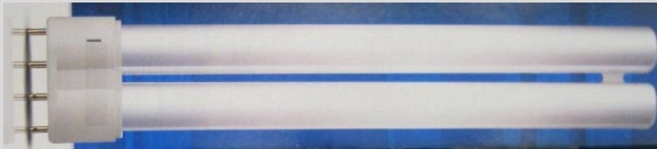
4-pin "PL" type lamp. Can be over 500 mm long, so there is a possibility to mistake it for a T-5 lamp. The lamp is distinguished by its connections being at one end, unlike T-5, and other linear tubes which have connections at each end.
