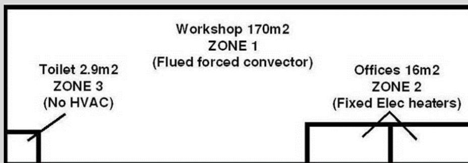
A separate zone must still be created to represent the differing activity of the toilet compared to the surrounding workshop zone. The message "**Warning: area seems small – are you sure?**" flags to the iSBEMie user that the entered zone area is small in case the user has made an error during the area input. Since the toilet is unheated, the walls to the toilet, as seen from the workshop, are subject to the guidance in Appendix 8 of the NEAP Survey Guide.
