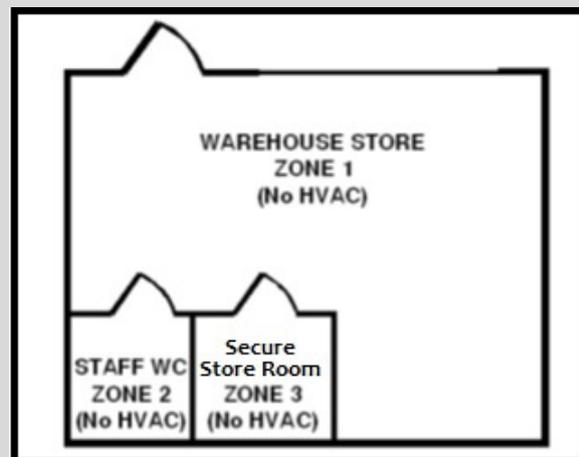
**Updated guidance:** Version iSBEMie 5.5h allows production of an XML without need to have a HVAC system in a model. The final model can be produced with the three zones set with "Zones without HVAC".
