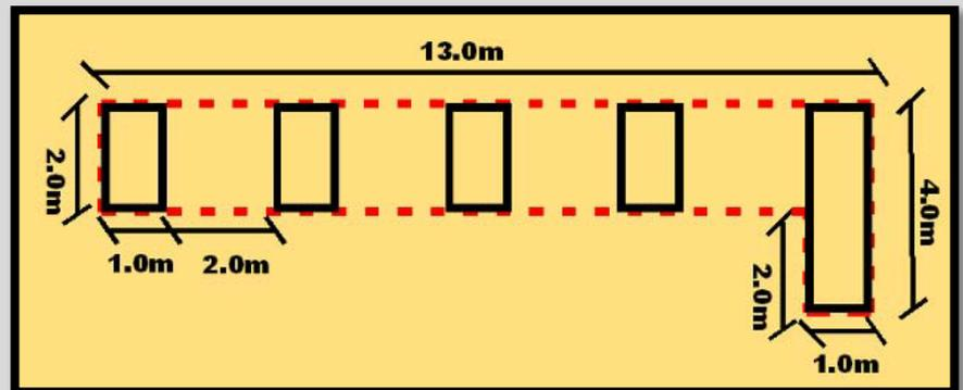
**Example 2: Rooflight area calculation**
