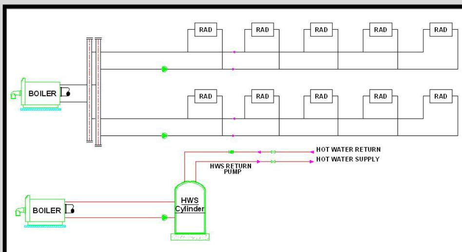
It is not correct to select “Dedicated hot water boiler” when the boiler also serves the space heating system, for example, the schematic below. In the case where the boiler is serving both the space heating and the hot water storage system, select “Same as HVAC”.
