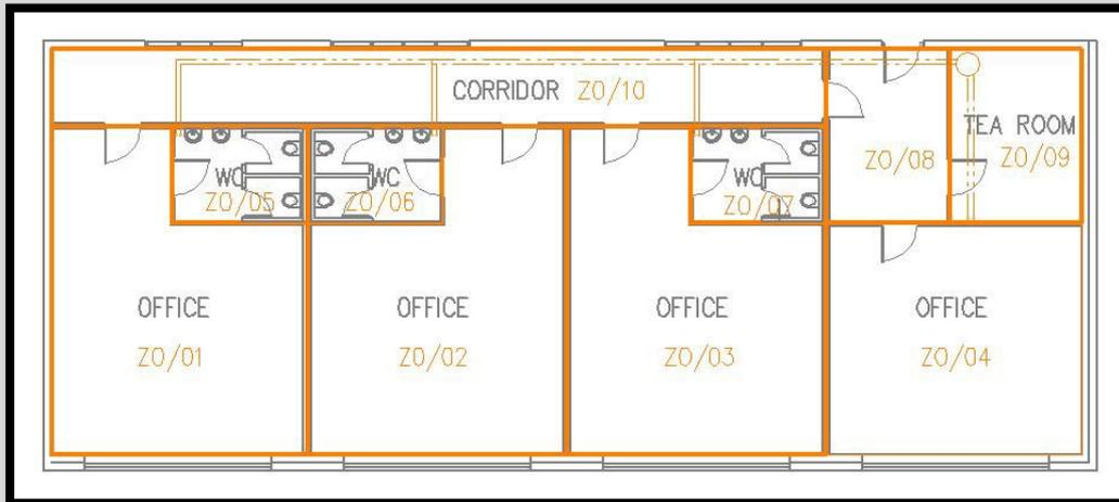
The assessor incorrectly assigned the actual HWS system (Installed HWS) to only the toilets and tea room, and a default HWS (Basic HWS) to the remainder of the zones:
