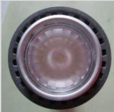
LED replacement for a tungsten spot lamp bulb.
