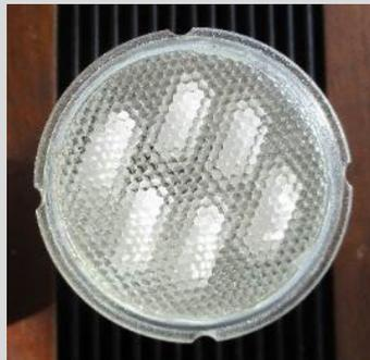
CFL replacement for a tungsten spot lamp bulb. These were an energy-saving alternative to tungsten spotlight bulbs, but have mostly been surpassed by LEDs. They can still be found in existing buildings but are unlikely to be included in a new lighting installation.
