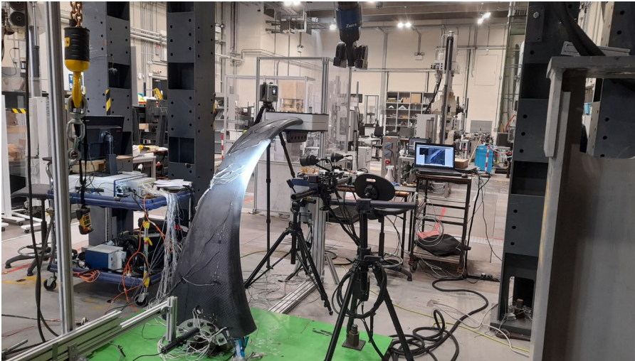
Figure 1 Composite test specimen being tested at the University of Galway Large Structures Test Laboratory
