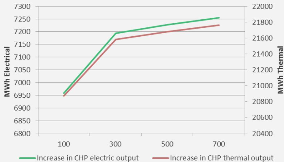
Figure 6: Optimising Size of Thermal Storage
