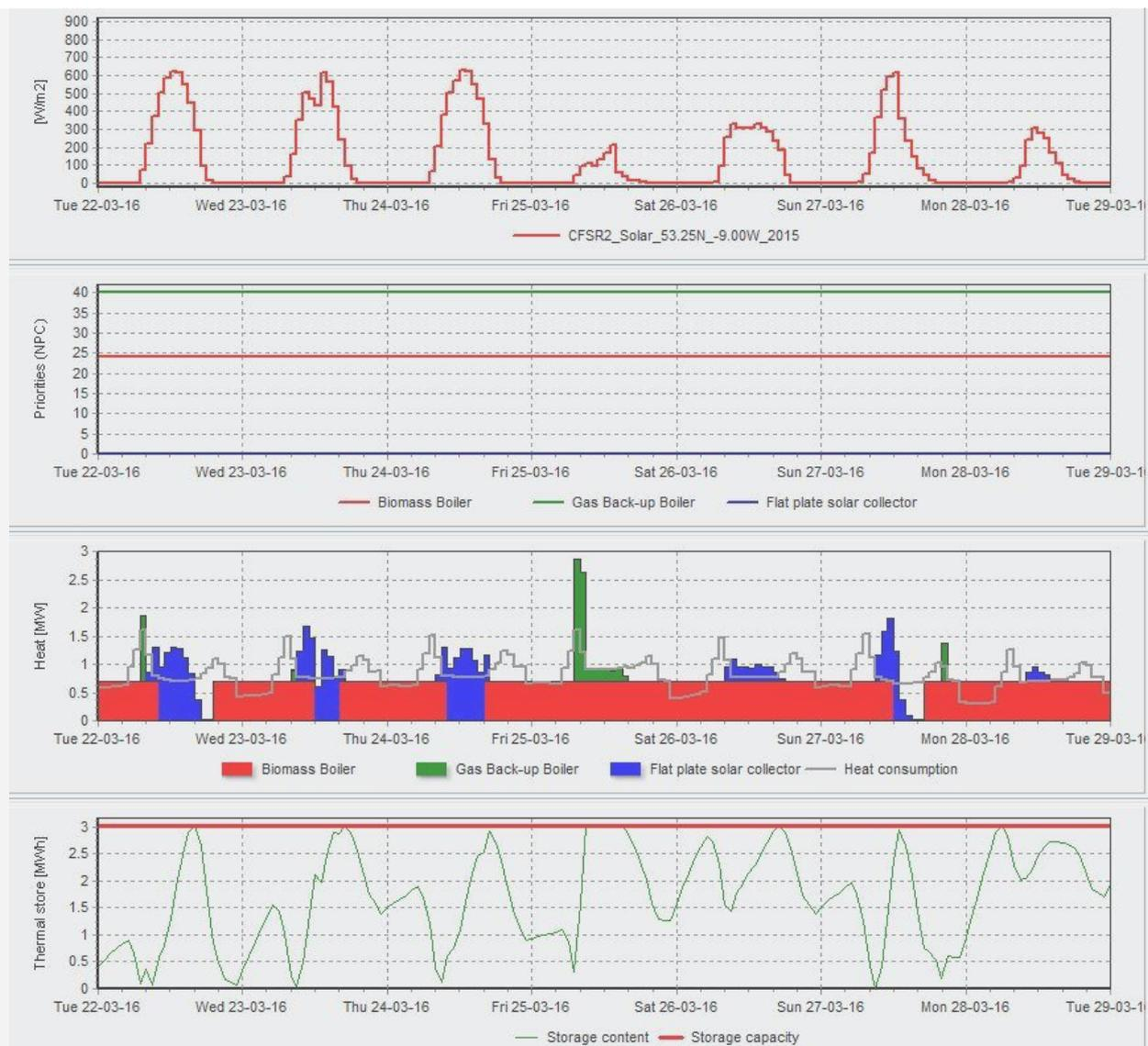
Figure 23: Production Graphic; Solar Collectors, Biomass Boiler and Gas Back-up Boilers
