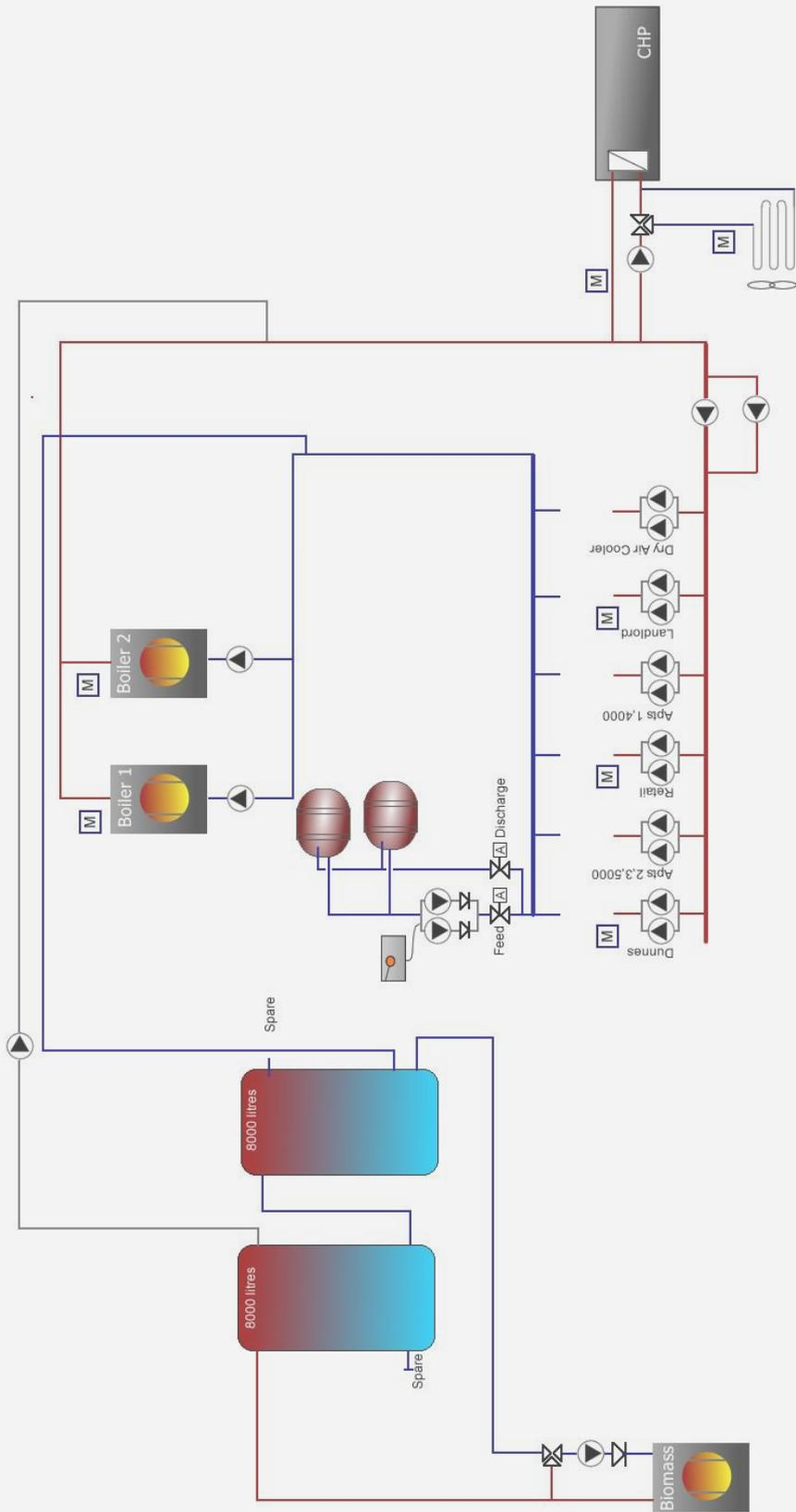
Figure 33: Process diagram for energy centre (Kaizen energy)
