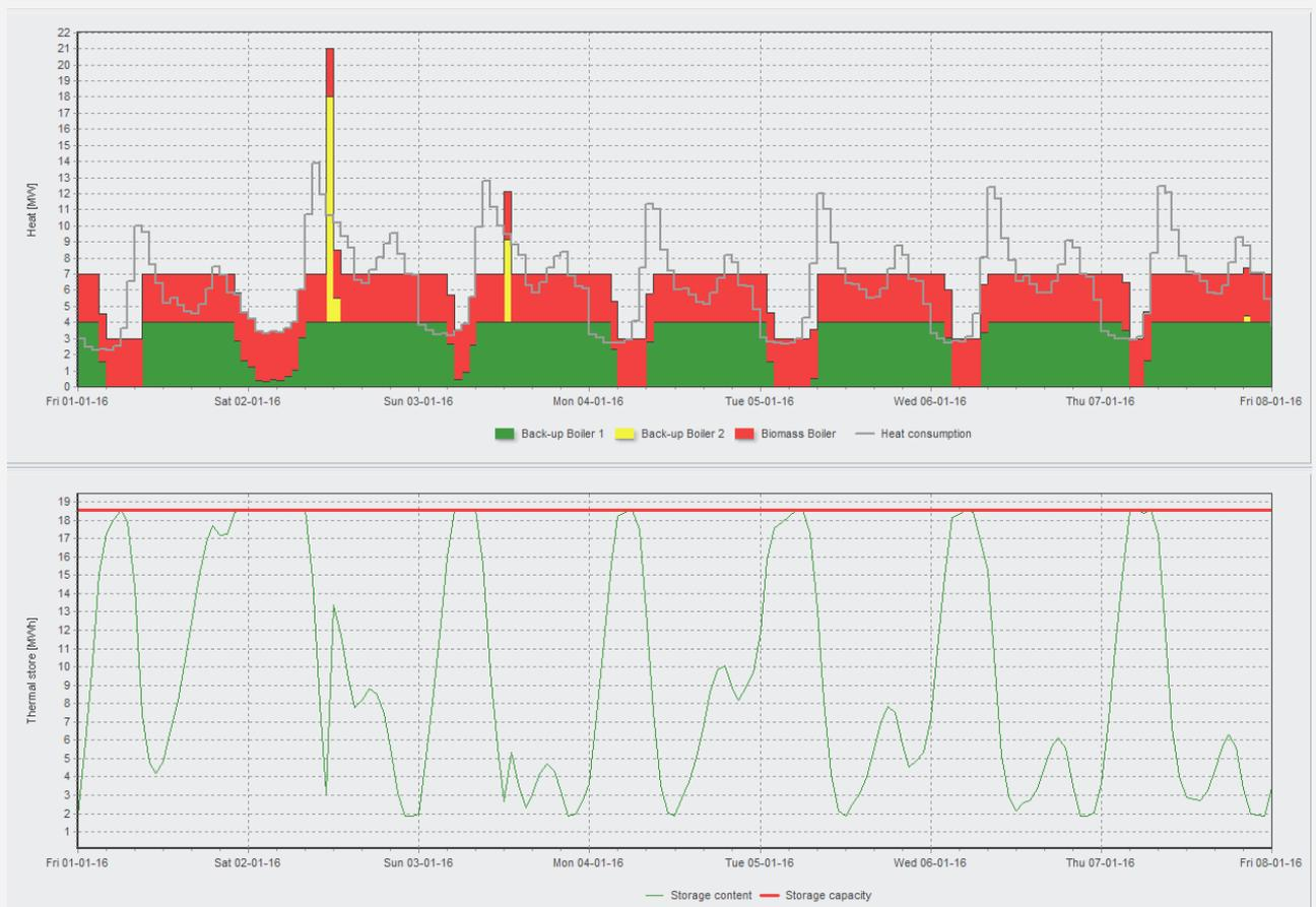
Figure 12: Production Graphic; Biomass boiler, back-up boilers, thermal storage
