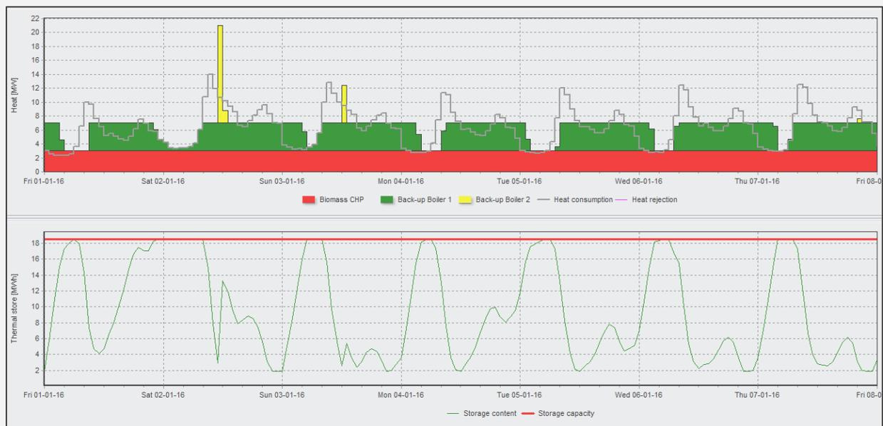
Figure 7: Production graphic; CHP, back-up boilers and thermal store
