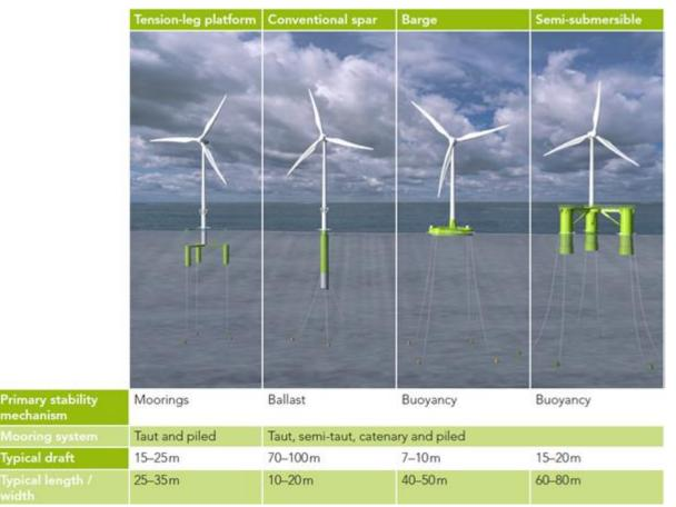
Figure 5-5: Summary of the varying floater platform types and mooring systems
