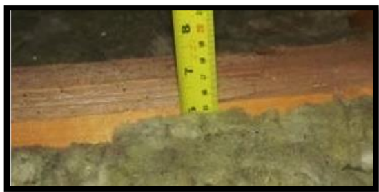
Figure 6.1: Measuring roof insulation thickness
