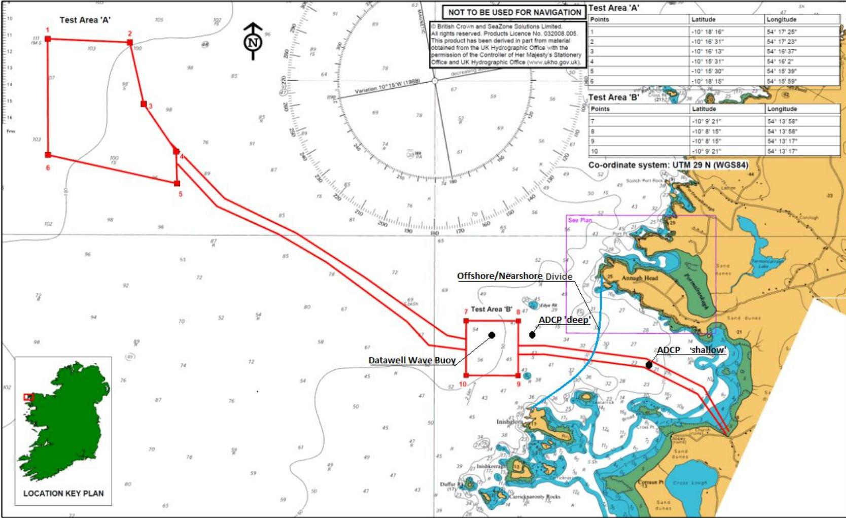
Figure 3.1 Wave and Current Measurement locations
