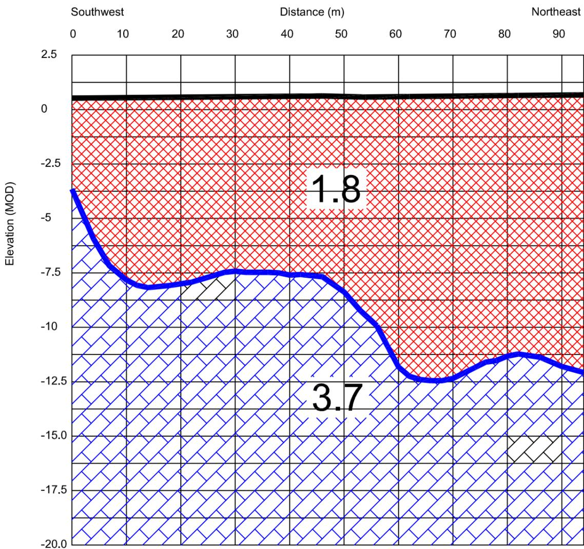
Seismic Refraction Profiles S19 & S20 Model
