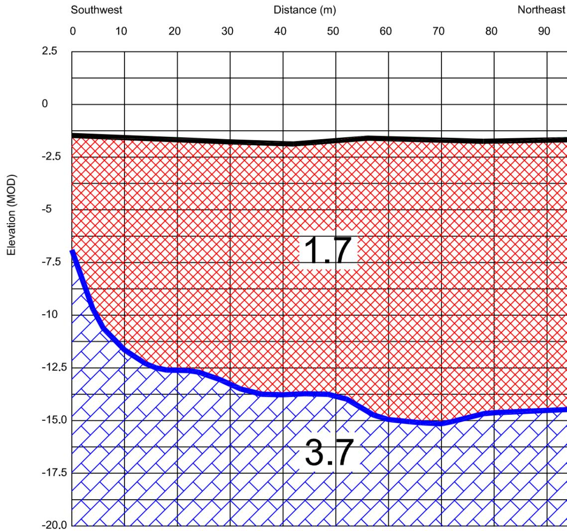
Seismic Refraction Profiles S5 & S6 Model
