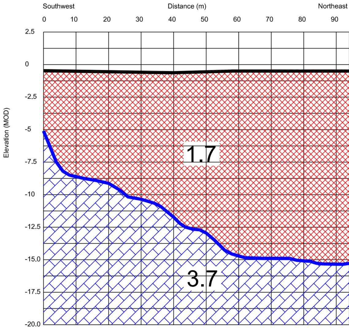
Seismic Refraction Profiles S9 & S16 Model
