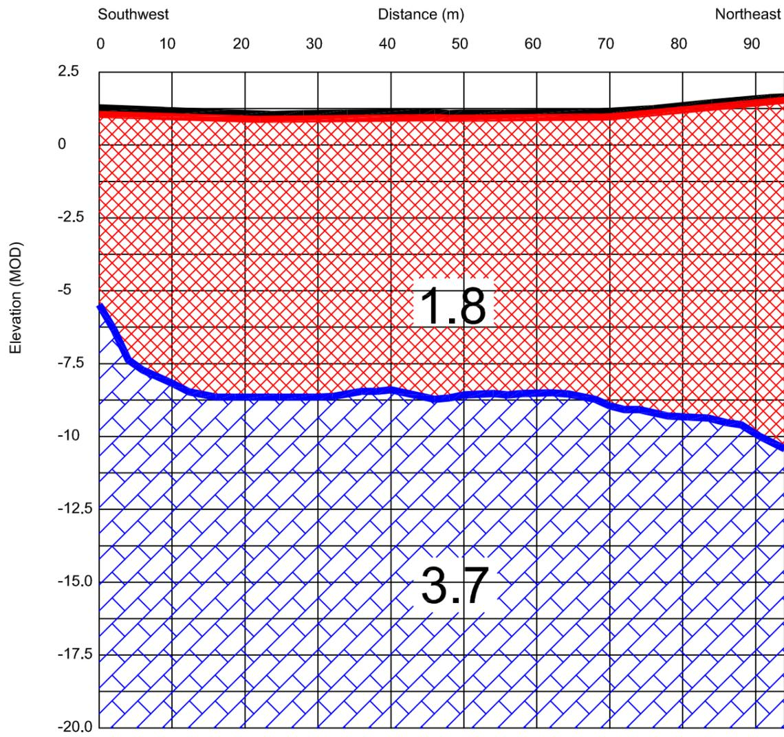
Seismic Refraction Profiles S10 & S11 Model
