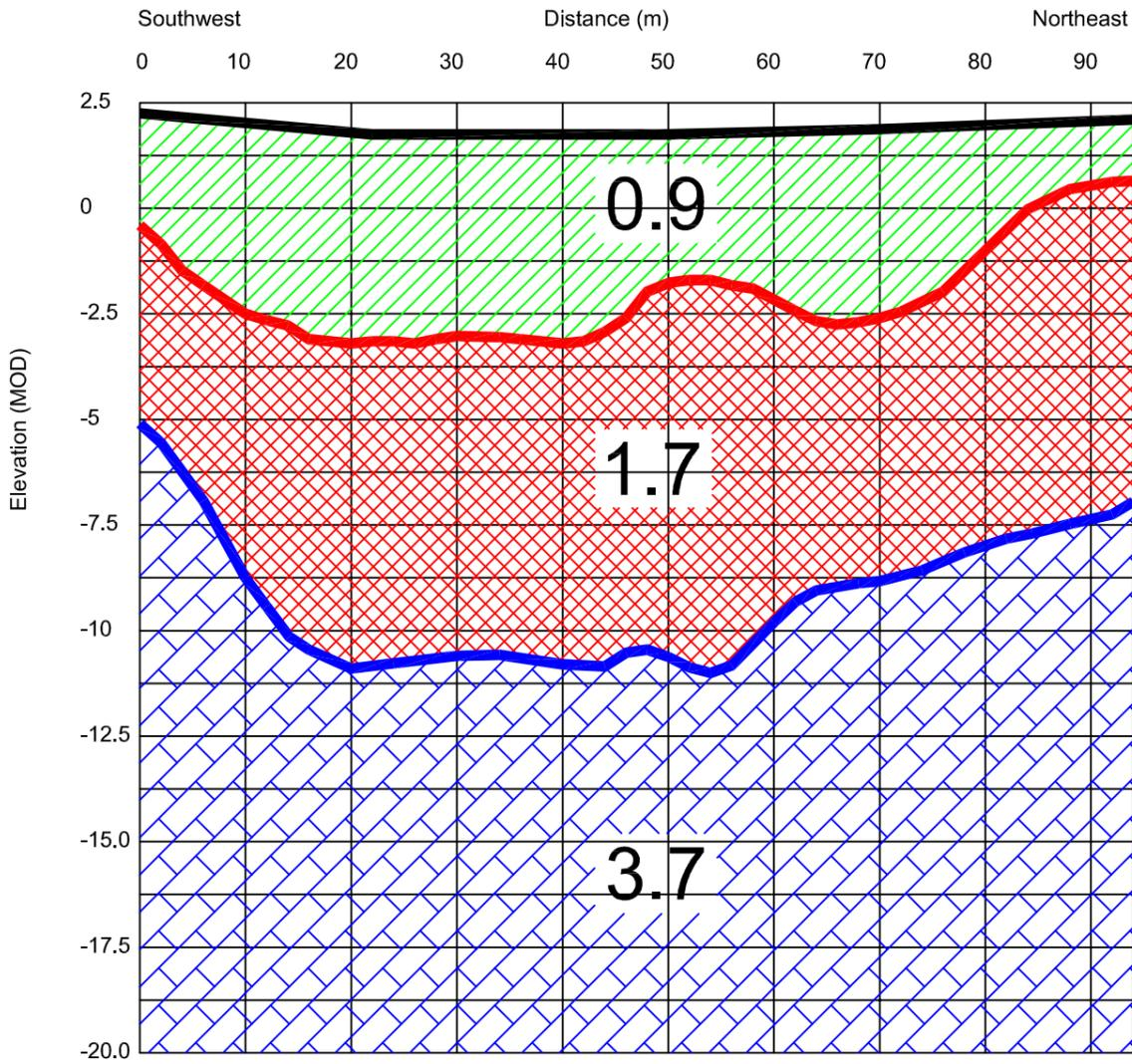
Seismic Refraction Profiles S14 & S15 Model
