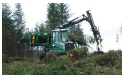
Timberjack bundler in operation at a Coillte site, Fermoy, Co. Cork
