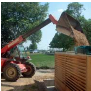
Figure 1 - The loading of the silo with wood chips using normal farm vehicles.
